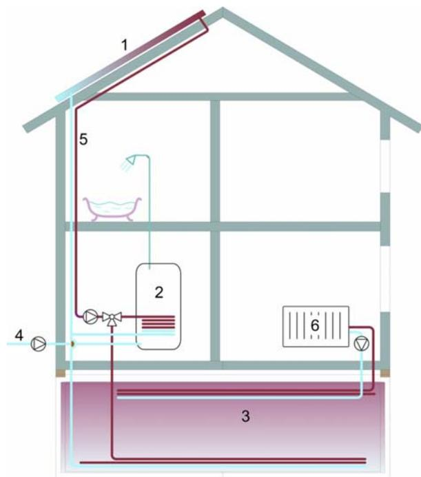
Fig. 1. Diagram of a house with solar thermal collectors and a thermal storage unit installed under the house.
