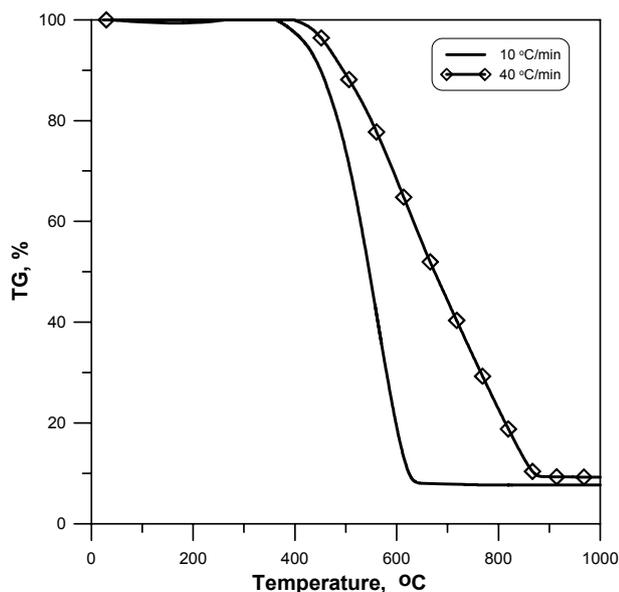
Fig. 5. TG curves for coal at heating rate 10°C/min and 40°C/min under air atmosphere.
