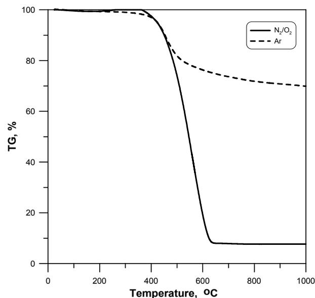
Fig. 4. TG curves for coal at  $10^\circ\text{C}/\text{min}$  heating rate under air ( $\text{N}_2/\text{O}_2$ ) and argon (Ar) atmospheres.
