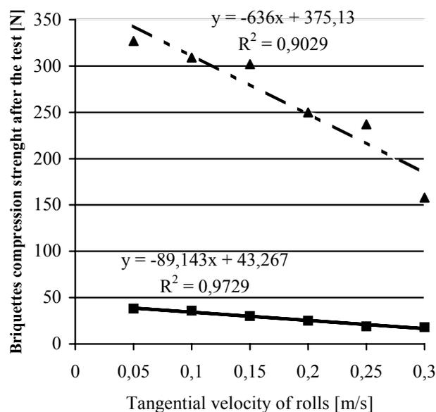
Fig. 3. Graphical expression of dependence of briquette compression strength after the test in relation to the tangential velocity of rolls.
