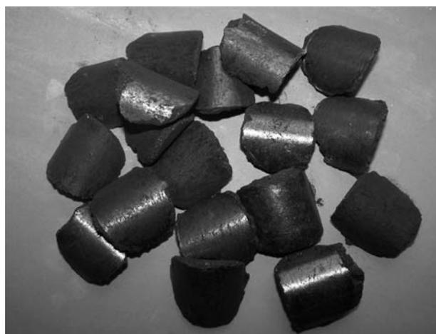
Fig. 1. Saddle-shaped briquettes with a volume of 6.5 cm<sup>3</sup>, obtained in a laboratory LPW 450 roll press, made of fine coking coal.
