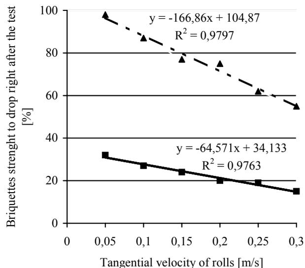
Fig. 2. Graphical expression of dependence of briquette strength to drop right after the test in relation to the tangential velocity of rolls.
