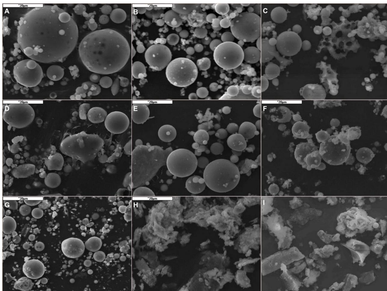
Fig. 1. Micrograph of fly ash: A-P1, B-P2, C-PB1, D-PB2, E-PB3, F-PS, G-PSB, H-FS, I-FSB.
