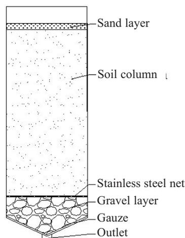
Fig. 2. Experimental design of soil column.
