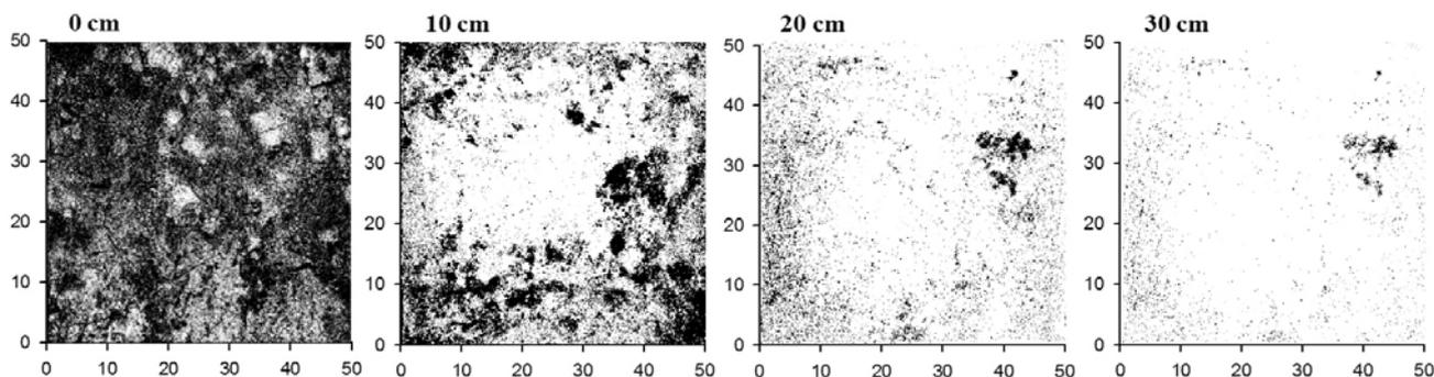
Fig. 3. Image of preferential pathways distribution in horizontal direction.
