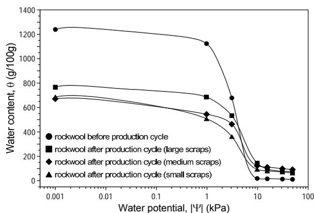
Fig. 3. Moisture characteristics curve of rockwool before and after production cycle.
