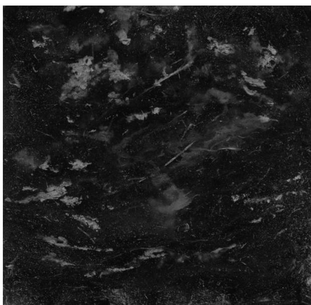
Fig. 1. Structure of the rockwool waste (large scraps 5×5 cm in size). Image size 8×9 cm.
