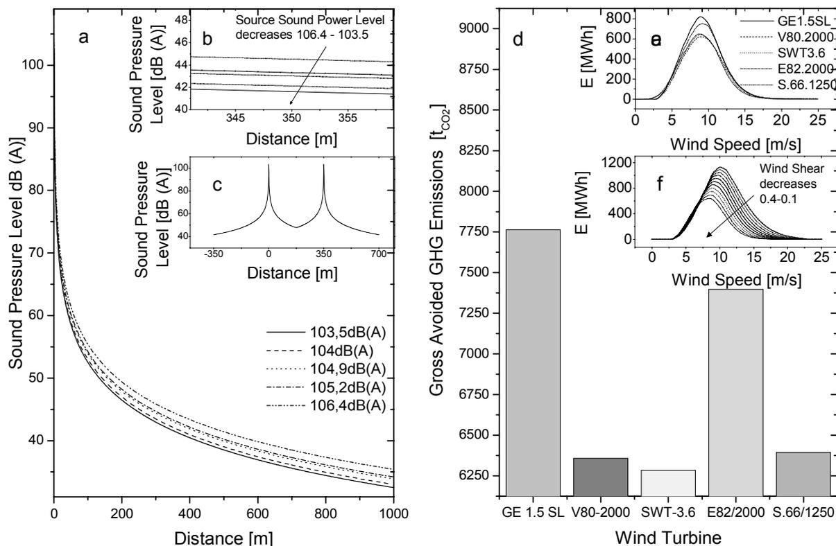
Fig. 1. Damping of sound pressure level with distance for analyzed wind turbines (a). Decrease of sound pressure level with distance in a free field at range of distance 340-360 m (b). Changing of sound pressure level vs. distance between two wind turbines (c). The gross avoided GHG emission for various wind power plants (d). The quantity of energy produced from different types of wind turbines for identical wind conditions (e). The quantity of energy produced for a wind shear range 0.1-0.4 (f).
