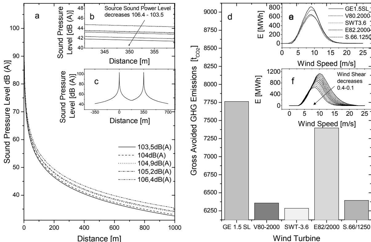
Fig. 1. Damping of sound pressure level with distance for analyzed wind turbines (a). Decrease of sound pressure level with distance in a free field at range of distance 340-360 m (b). Changing of sound pressure level vs. distance between two wind turbines (c). The gross avoided GHG emission for various wind power plants (d). The quantity of energy produced from different types of wind turbines for identical wind conditions (e). The quantity of energy produced for a wind shear range 0.1-0.4 (f).
