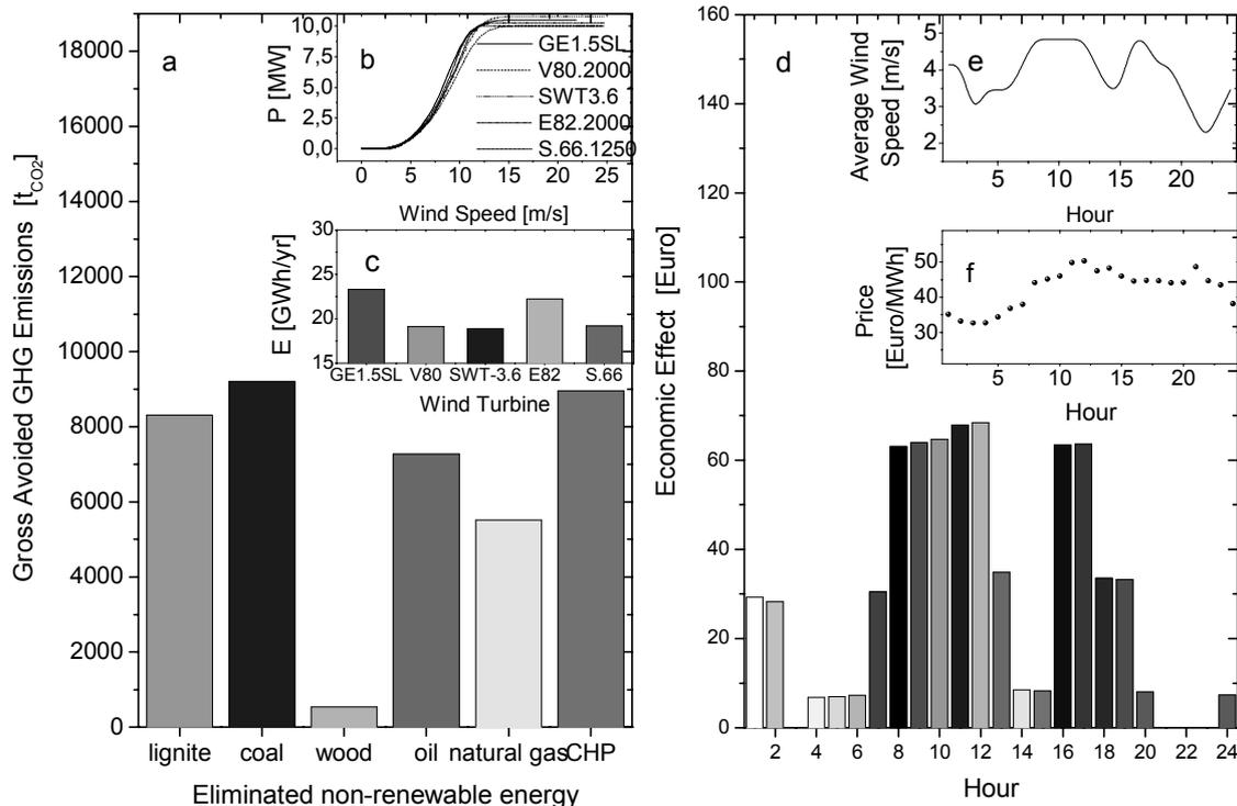
Fig. 2. Environmental effects of a functioning system (a). Power curve of analyzed wind power plants (b). The amount of energy produced annually by power plants (c). Economic effect of a wind turbine for a select period of time (d). Average wind speed distribution for chosen location (e). Price of energy on energy stock (f).
