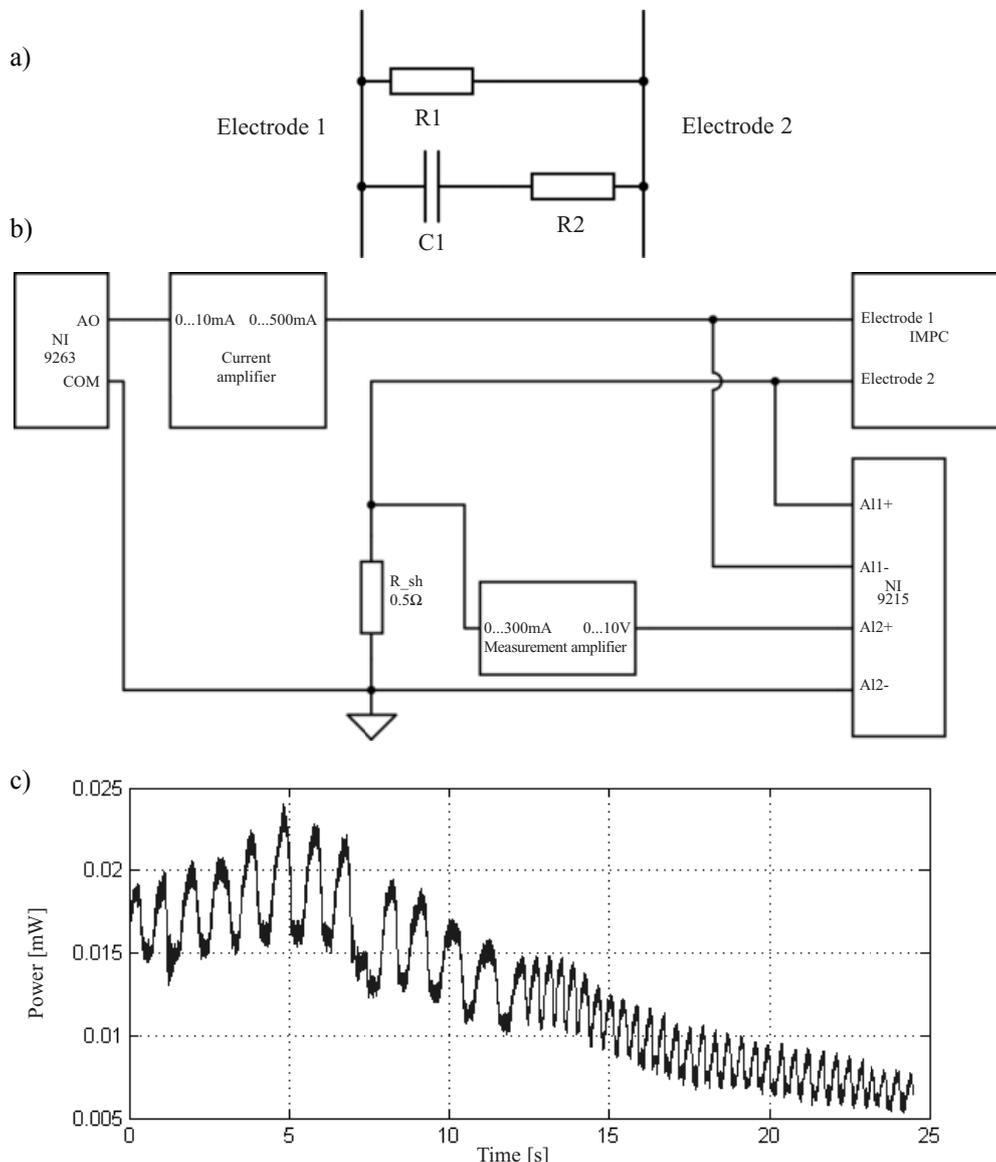
Fig. 1. IPMC modelling: a) equivalent electrical circuit of the IPMC, b) signal generation and data acquisition circuitry, c) time-domain signal from data acquisition card (IPMC power generation capabilities).
