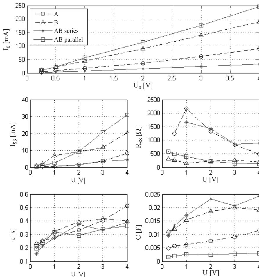
Fig. 2. Relationships between actuation voltage  $U$  and:  $I_0$  – maximum charging current,  $I_{SS}$  – steady state current,  $R_{SS}$  – steady state resistance,  $\tau_s$  – time constant,  $C$  – capacity.
