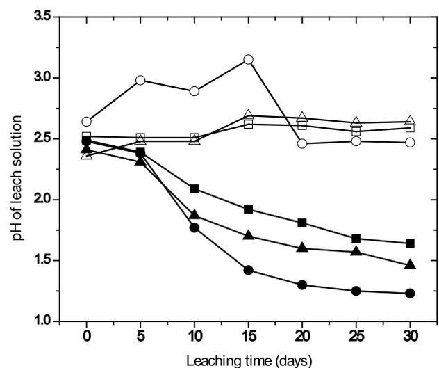
Fig. 6. a) pH and b) redox potential profiles of leach solutions obtained from various pulp densities of copper ore with isolated strain of acidophilic iron- and sulfur-oxidizing bacteria; symbol designations:  $\square$  = control 5% (w/v),  $\blacksquare$  = inoculated 5% (w/v),  $\triangle$  = control 10% (w/v),  $\blacktriangle$  = inoculated 10% (w/v),  $\circ$  = control 20% (w/v) and  $\bullet$  = inoculated 20% (w/v).
