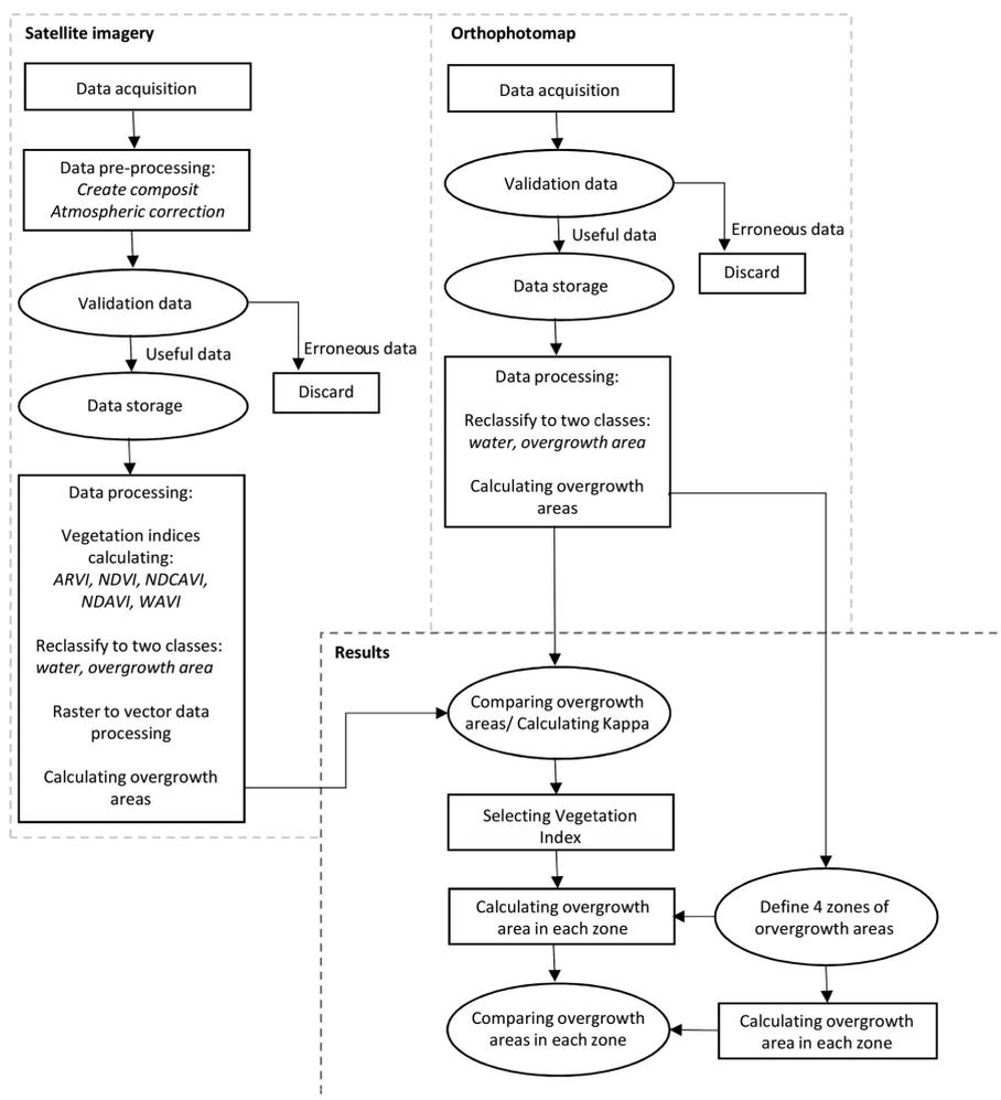
Fig. 2. Flow chart for remote sensing data analysis.
