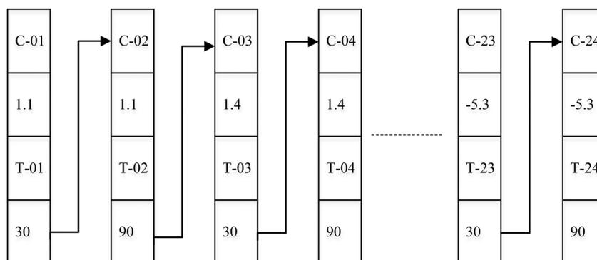
Fig. 3. Demonstration of settings for the rapid temperature experiment chamber as used in the variable temperature regime (VTR) treatment for measuring mollisol aggregate stability in northeastern China (C-01: the first section desired temperature, T-01: the time from current measured value temperature to the first section desired temperature, C-02: the first section desired temperature, T-02: the time of keeping the constant desired temperature).
