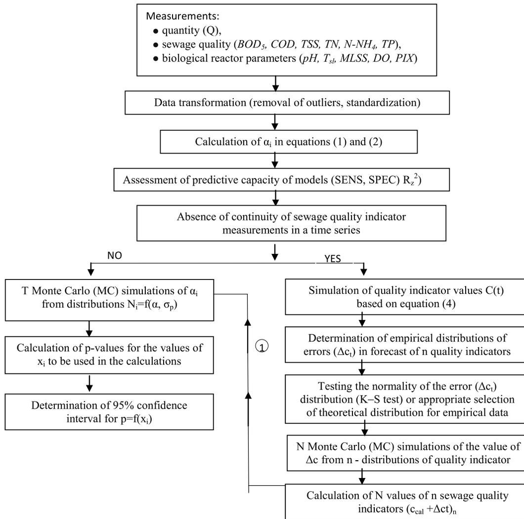
Fig. 1. Calculation diagram of the influence of parametric uncertainty and uncertainty of forecast of wastewater quality indicators on SVI simulation by classification models.
