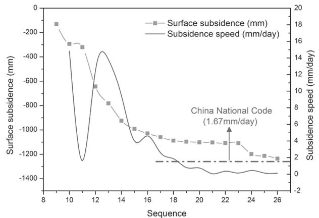
Fig. 5. Surface subsidence and subsidence speed curves of no. 17 point.
