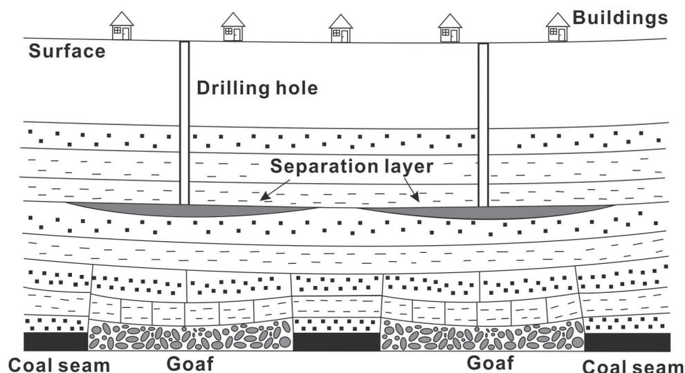
Fig. 1. Diagrammatic sketch of Backfilling in Separation.
