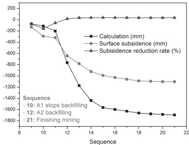
Fig. 6. Surface subsidence curves of calculation and observation of no. 17 point.
