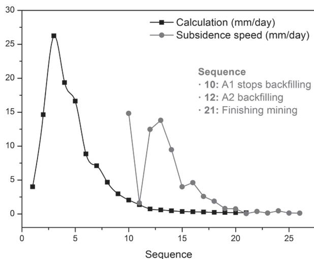
Fig. 7. Surface subsidence speed curves of calculation and observation of no. 17 point.
