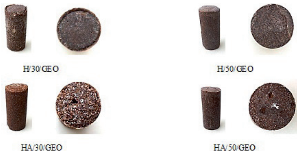
Fig. 1. Geopolymers obtained from raw halloysite (H/30/GEO, H/50/GEO) and activated halloysite (H/30/GEO, H/50/GEO).
