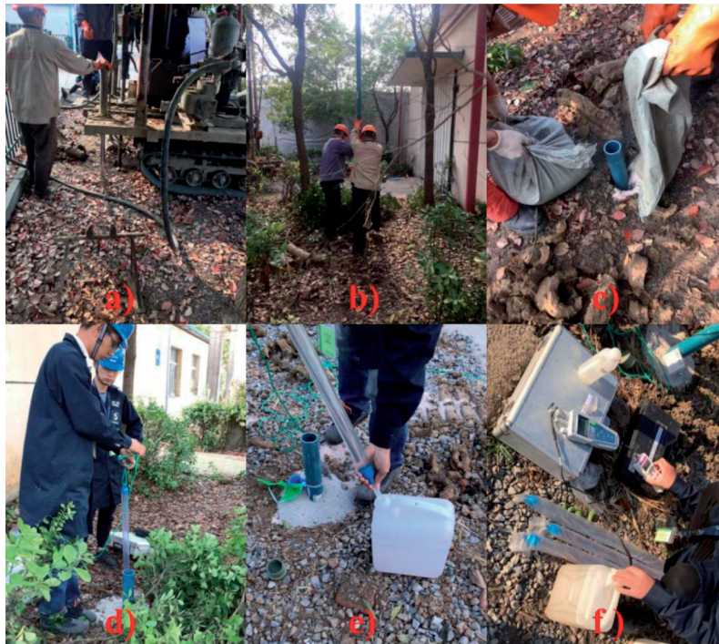
Fig. 2. Field test photos a) Drilling, b) Installing PVC pipe, c) Filling with filter material, d) Washing well before sampling, e) Sample collection, and f) Parameter determination.
