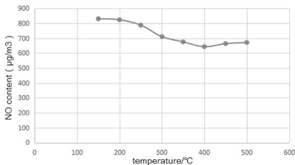
Fig. 7. The variation curve of NO content after the catalytic.
