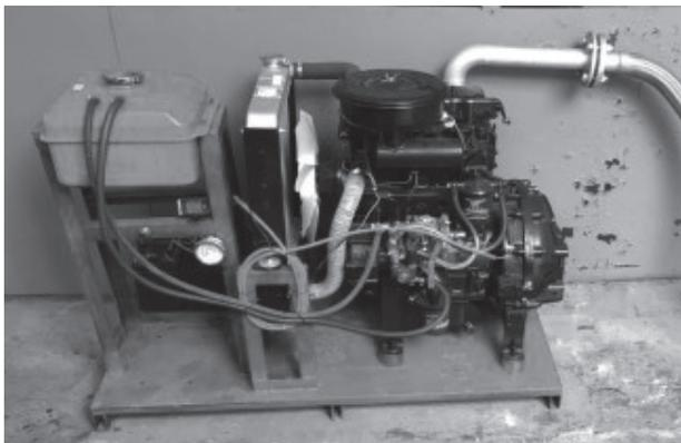
Fig. 4. Changchai CZ2102 diesel engine.
