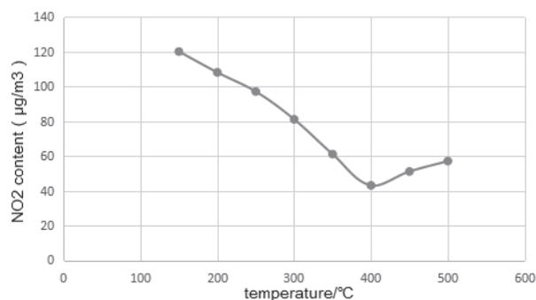
Fig. 8. The variation curve of NO<sub>2</sub> content after the catalytic.
