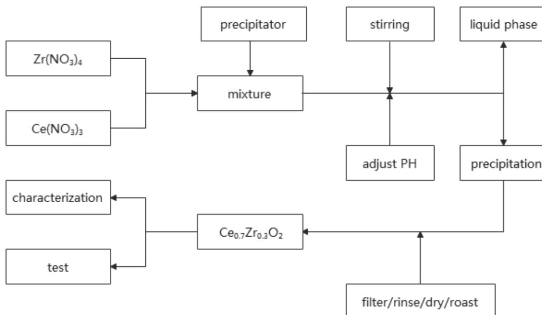
Fig. 1. Preparation flowchart of cerium-zirconium composite oxides.
