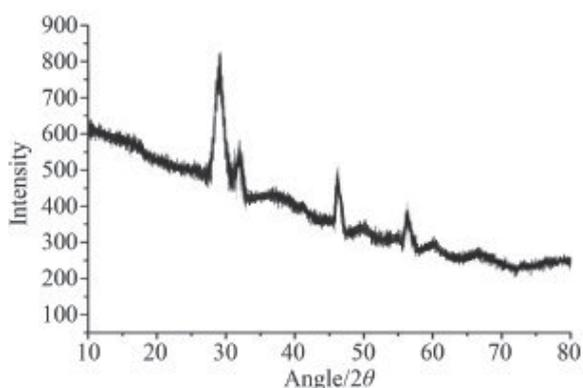
Fig. 2. XRD image of cerium-zirconium composite oxides.
