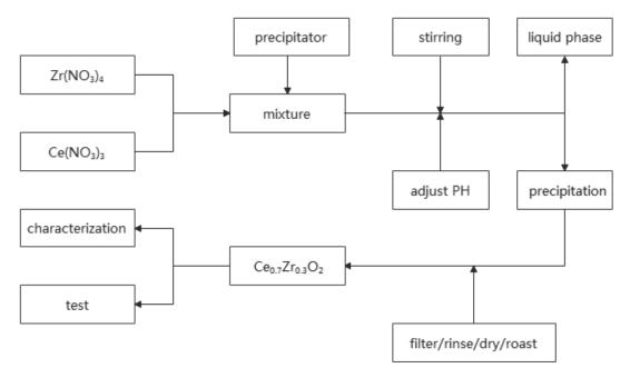
Fig. 1. Preparation flowchart of cerium-zirconium composite oxides.
