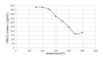
Fig. 5. The variation curve of PM2.5 content after the catalytic.
