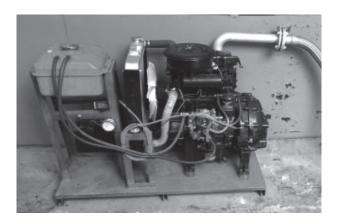
Fig. 4. Changchai CZ2102 diesel engine.
