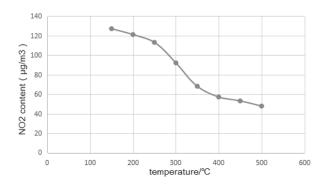
Fig. 12. The variation curve of NO<sub>2</sub> content after the catalytic.
