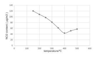
Fig. 8. The variation curve of NO<sub>2</sub> content after the catalytic.
