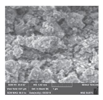
Fig. 3. SEM image of cerium-zirconium composite oxides.
