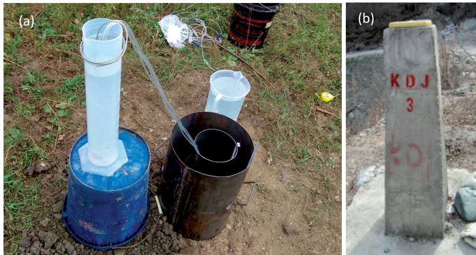
Fig. 4. Field monitoring a) Double-Ring Permeability test; b) Monitoring station.
