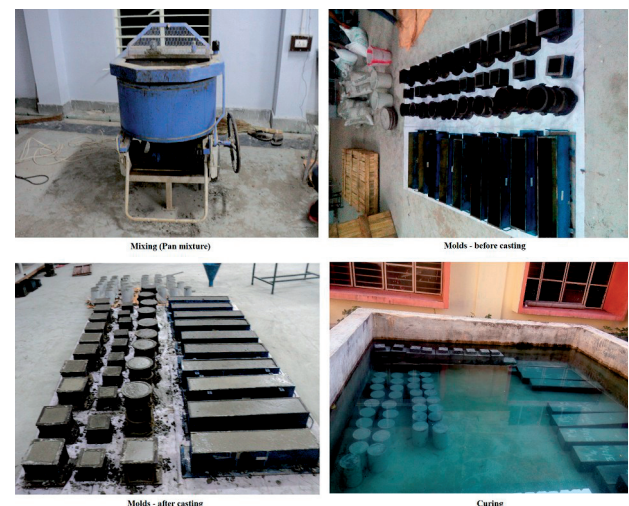
Fig. 2. Mixing, casting and curing of HPC.
