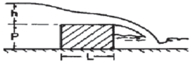
Fig. 1. Schematic design of rectangular broad-crested weirs (Hager & Schwalt, 1994).
