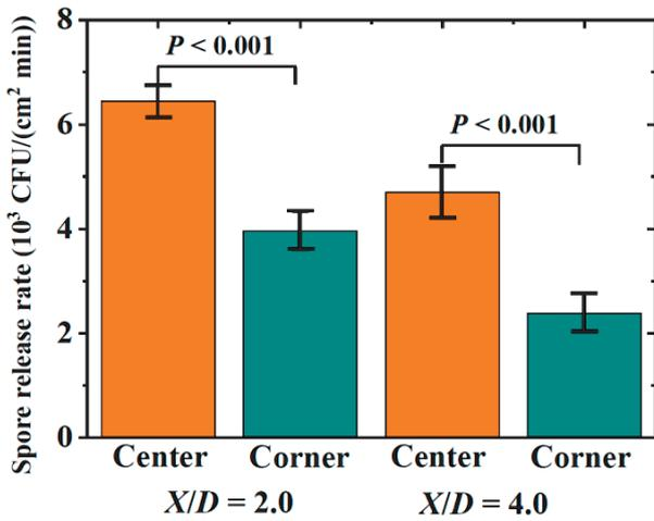
Fig. 3. Spore release rate of the colony at different positions on the bottom surface of the rectangular duct when the inlet air speed was 5.00 m/s, where error bars represent the standard deviations of five repeated experiments.
