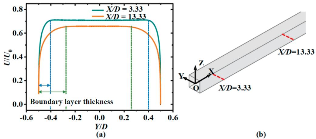
Fig. 7. Effect of the  $Y/D$  value on the air speed distribution at the height of the colony on the inner surface of the rectangular duct: a) variation of the local dimensionless air speed ( $U/U_0$ ) with the  $Y/D$  value at different dimensionless displacement ( $X/D$ ) values under the inlet air speed of 6.00 m/s; b) schematic diagram of the location of the colony for different dimensionless displacements.
