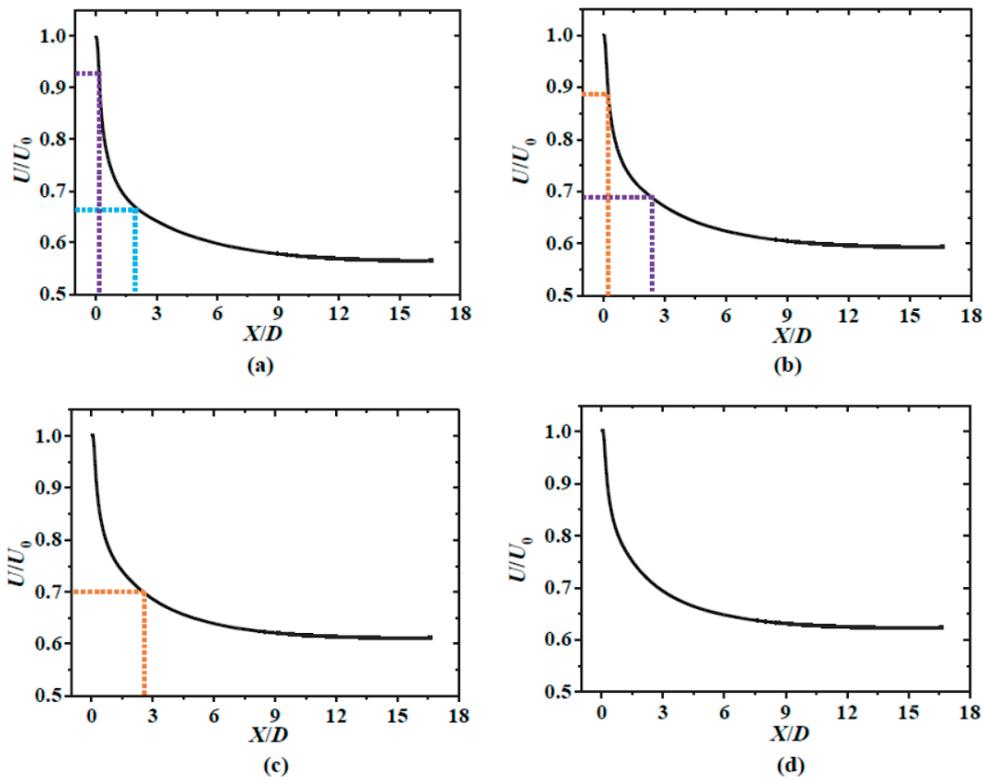
Fig. 4. Variation of the local dimensionless air speed ( $U/U_0$ ) at the height of *A. niger* spores with the dimensionless displacement ( $X/D$ ) under different inlet air speeds: a) 3.00 m/s; b) 4.00 m/s; c) 5.00 m/s; d) 6.00 m/s.
