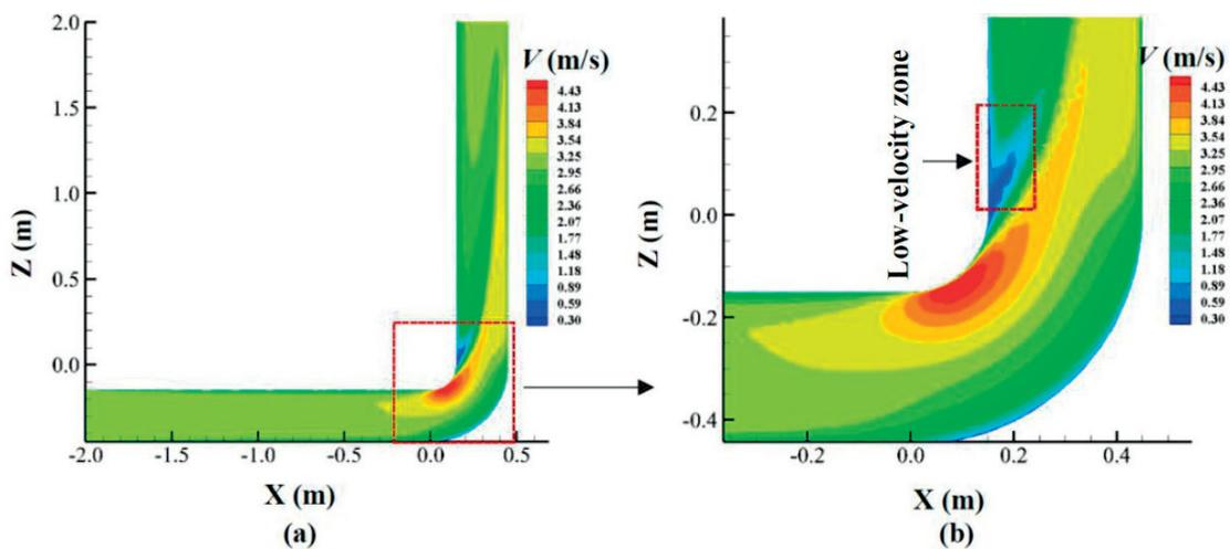
Fig. 8. Velocity distribution of the airflow in the elbow duct under the inlet air speed of 3.00 m/s when the  $\beta$  value was 1.0: a) planar view; b) local enlarged view of the dotted area of the elbow.
