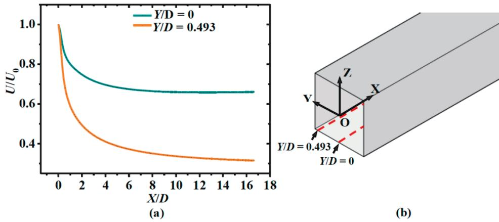
Fig. 6. Effect of the  $Y/D$  value on the air speed distribution at the height of the colony on the inner surface of the rectangular duct: a) variation of the local dimensionless air speed ( $U/U_0$ ) with the dimensionless displacement ( $X/D$ ) at different  $Y/D$  values under the inlet air speed of 6.00 m/s; b) schematic diagram of the location of the colony for different  $Y/D$  values.
