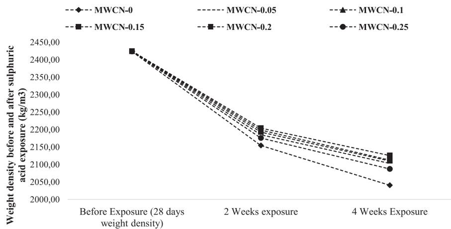
Fig. 4. Weight density before and after exposure to sulphuric acid.
