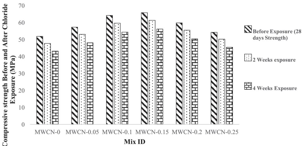
Fig. 3. Compressive strength before and after exposure to chloride solution.
