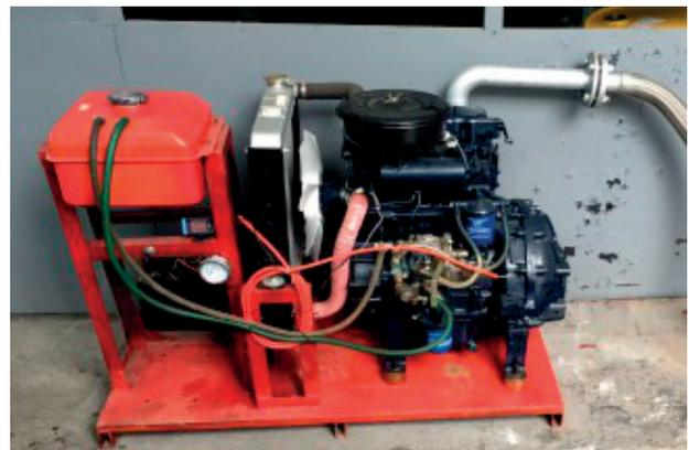
Fig. 10. Experimental platform of Changchai CZ2102 diesel engine.
