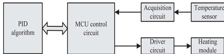
Fig. 2. Schematic diagram of temperature control scheme.
