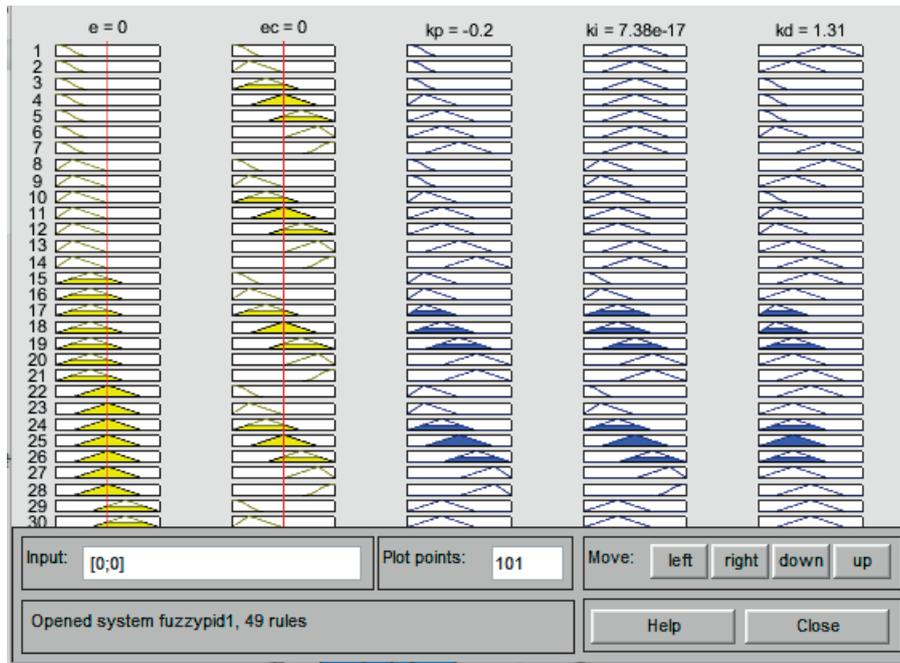
Fig. 10. FA-PID control rules.
