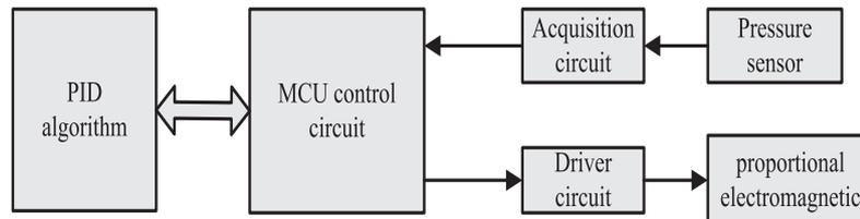
Fig. 3. Schematic diagram of pressure control scheme.
