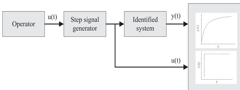
Fig. 4. Schematic diagram of system identification experiment.
