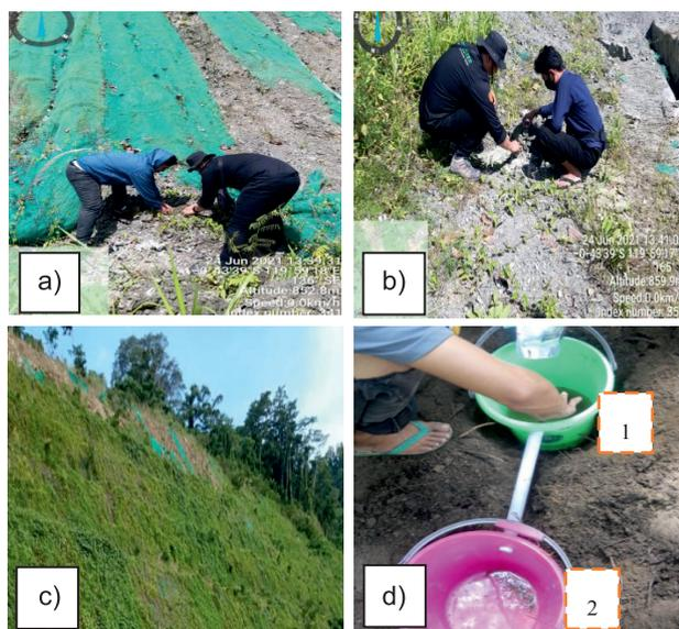
Fig. 2. Location of plot placement; a) geonet, b) geogrid, c) vegetation cover, d) bucket observations surface flow and erosion; (1) bucket 1, (2) bucket 2
