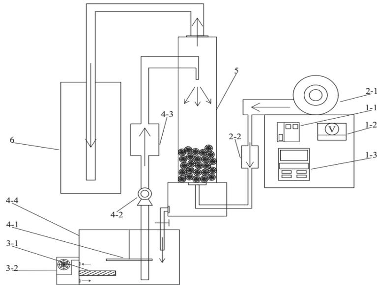
Fig. 1. Schematic diagram of ammonia nitrogen stripping device.
