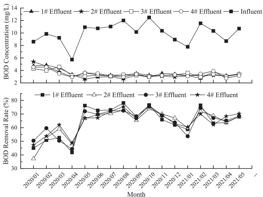
Fig. 4. BOD<sub>5</sub> in the influent and effluents of the SSFCW system and the corresponding removal rates.
