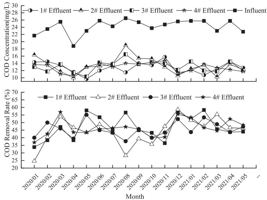
Fig. 3. COD<sub>Cr</sub> in the influent and effluents of the SSFCW system and the corresponding removal rates.
