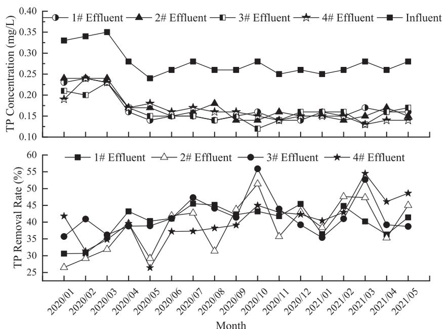
Fig. 6. TP in the influent and effluents of the SSFCW system and the corresponding removal rates
