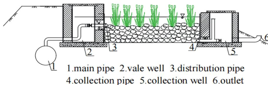
Fig. 2. The structure of the SSFCW unit.
