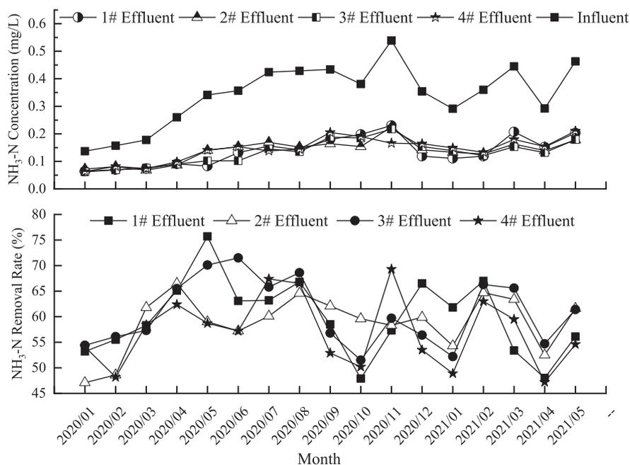
Fig. 5. NH<sub>3</sub>-N in the influent and effluents of the SSFCW system and the corresponding removal rates.
