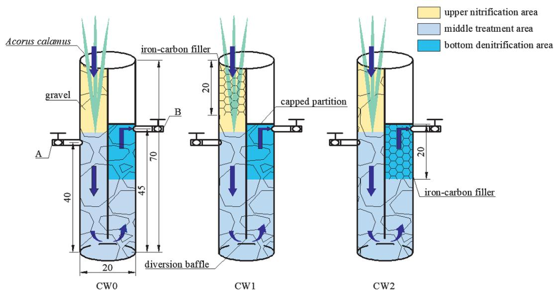
Fig. 1. Schematic diagram of the experimental CWs.
