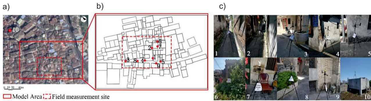
Fig. 3. Distribution of measured points. a) Study area and model area; b) field measurement site; c) pictures of the monitor site.
