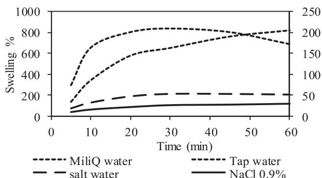
Fig. 4. The absorption capacity of SAP in water solutions with different salinities.
