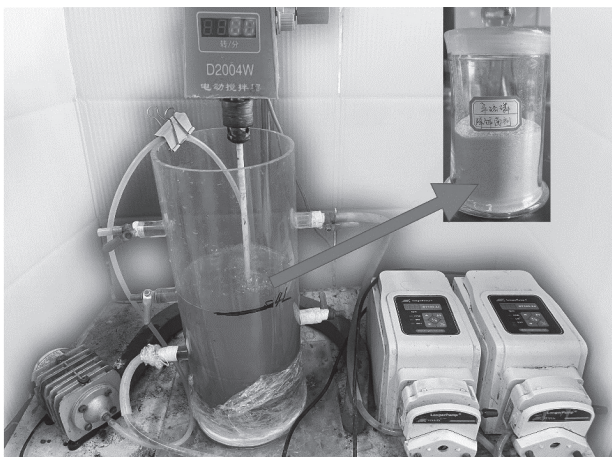
Fig. 1 The pesticide wastewater aeration biological treatment device with the application of the prepared microbial inoculum (insert: Physical map of the prepared microbial inoculum).
