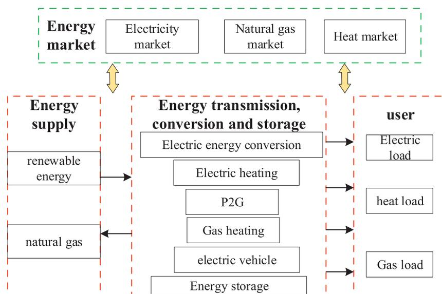
Fig. 1. Infrastructure of coupled gas-electric virtual power plants.
