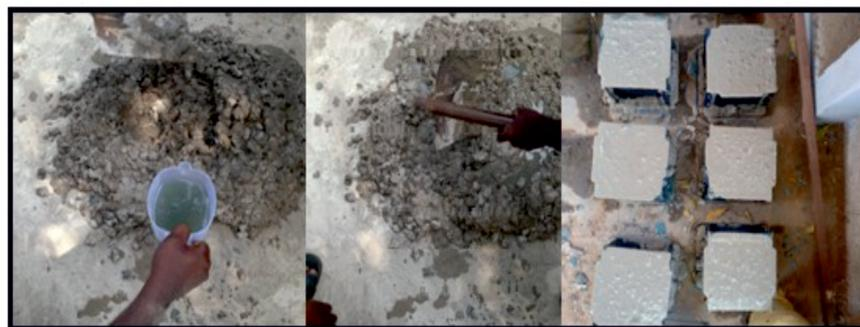
Fig. 4. Casting of Geo polymer Concrete.
