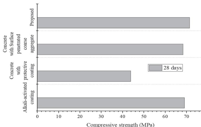
Fig. 8. Comparison of compressive strength at 28 days with existing methods.
