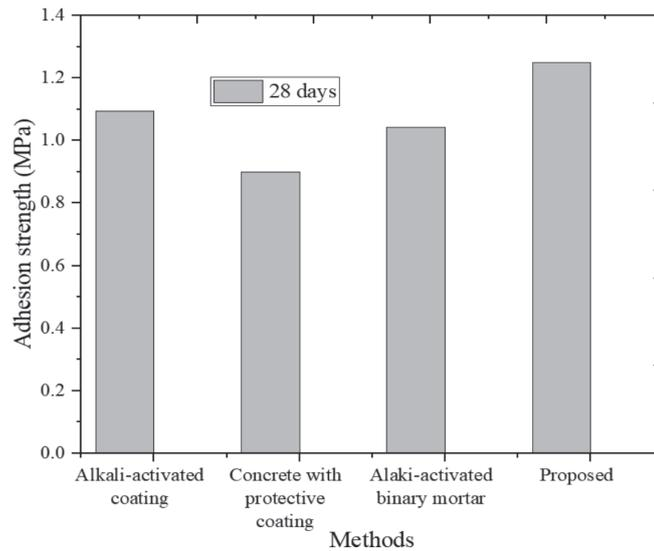
Fig. 9. Comparison of adhesion strength at 28 days with other methods.
