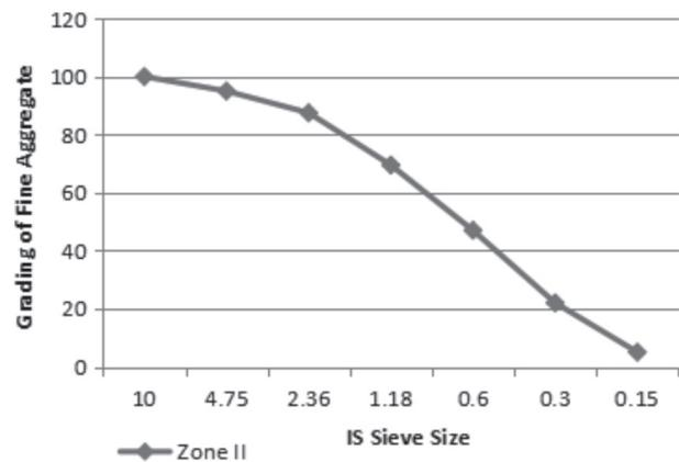
Fig. 2. Zone II - Grading Curve.
