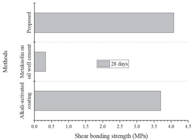
Fig. 10. Comparison of Shear bond strength at 28 days with other methods.
