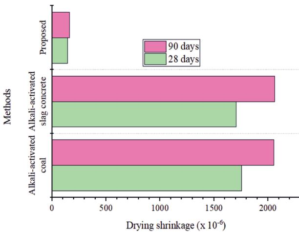
Fig. 11. Comparison of drying shrinkage.
