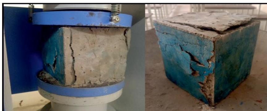
Fig. 5. Testing of Geo polymer Concrete.
