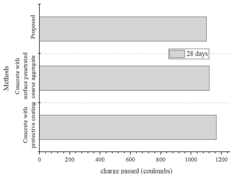
Fig. 13. Comparison of chloride permeability at 28 days.
