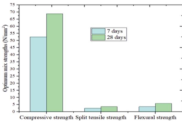
Fig. 6. Strengths of Optimum mix geopolymer concrete.
