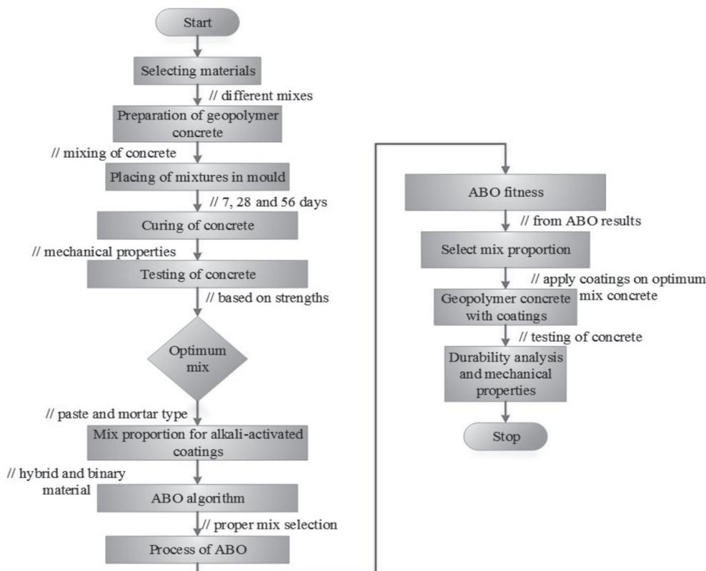
Fig. 7. Flow diagram of ABO algorithm in the selection of coating proportion.
