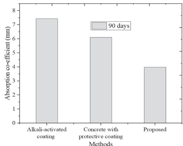
Fig. 12. Comparison of absorption co-efficient at 90 days.
