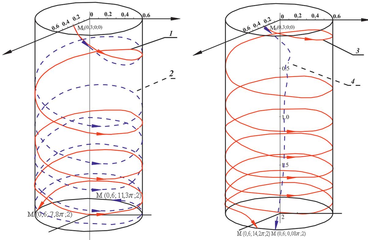
Fig. 2. At  $v_0 = 0$ , the trajectories of dust particles along the walls of the dust collector for various values of  $v_r$  and  $v_\varphi$ : 1)  $v_r = 45$  m/s and  $v_\varphi = 45$  m/s; 2)  $v_r = 32$  m/s and  $v_\varphi = 55$  m/s; 3)  $v_r = 0$  m/s and  $v_\varphi = 64$  m/s; 4)  $v_r = 63,99$  m/s and  $v_\varphi = 1$  m/s.
