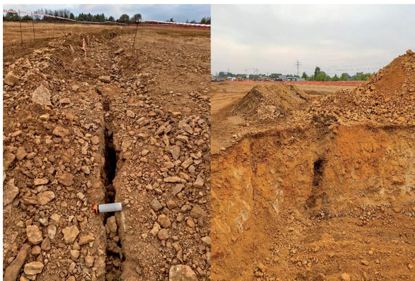
Fig.11. Discontinuous linear deformation along the North Fault in area B (copyright photo).
