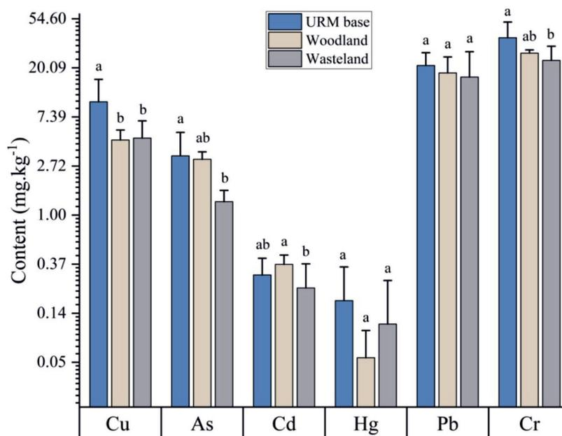
Fig. 3. Characteristics of heavy metal content in URM producing areas under different land use patterns. Note: Different lowercase letters indicate significant differences (P<0.05).
