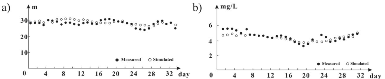
Fig. 4. Results of model tuning a) Comparison of measured and simulated water level values; b) Comparison of measured and simulated nitrate values.
