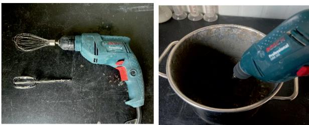
Fig. 6. Agitator and slurry mixing process.
