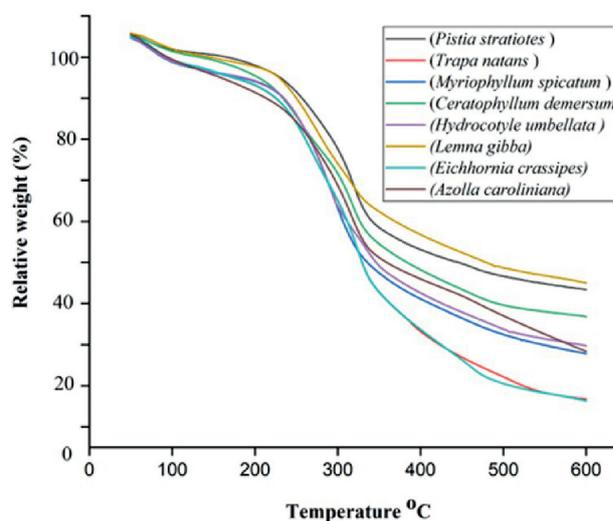
Fig. 1. Thermogravimetric analysis of biochar derived from different aquatic plants feedstock.
