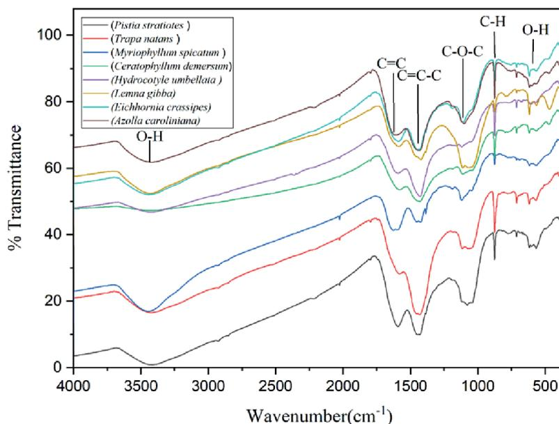
Fig. 2. FTIR spectra of biochars derived from different aquatic plants feedstock.
