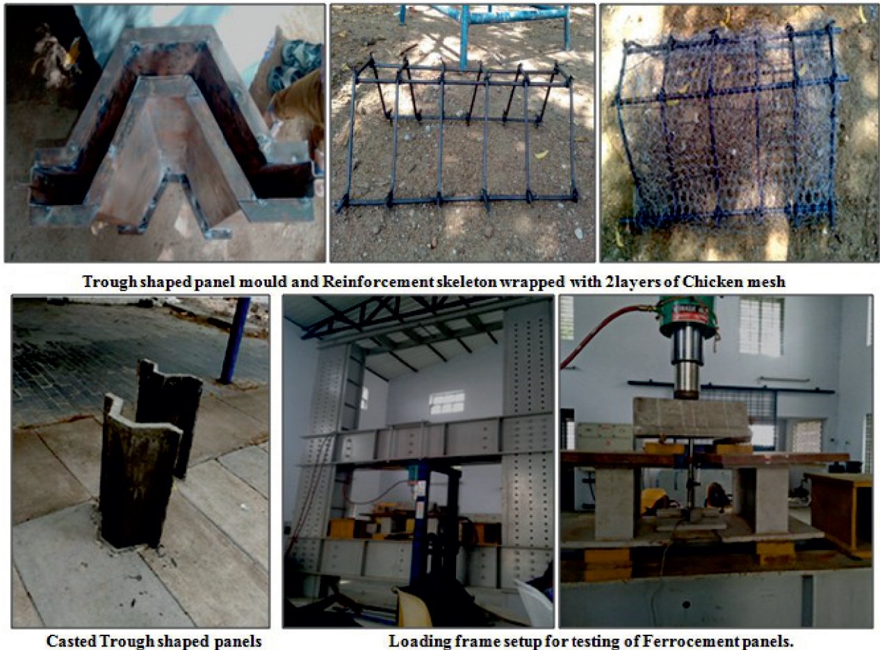
Fig. 1. Preparation, casting and testing of panels.
