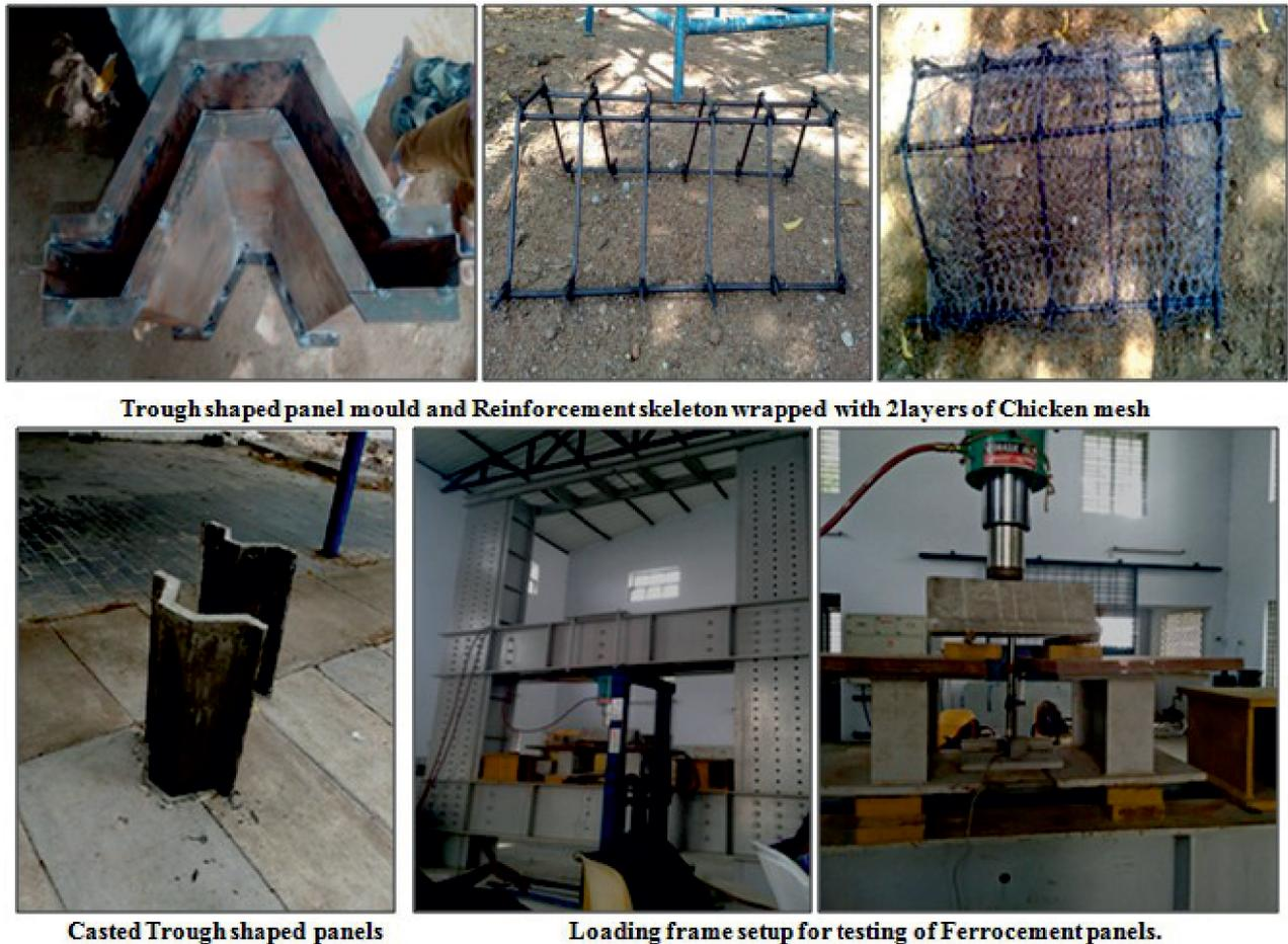
Fig. 1. Preparation, casting and testing of panels.
