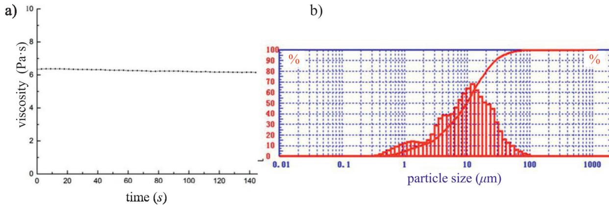
Fig 8. Feature of the grout: a) Viscosity change over time; b) Particle size distribution of cement.
