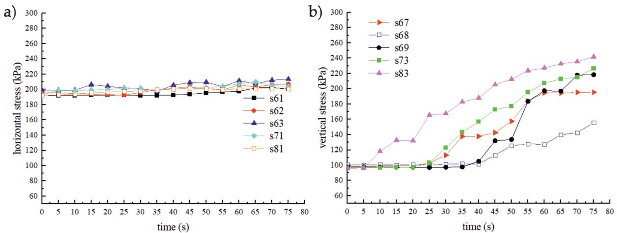
Fig. 11. Stress fluctuation of the first grouting: a) Horizontal stress by first grouting; b) Vertical stress by first grouting.
