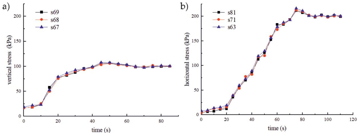
Fig. 10. Filling soil and place ground stress sensors: a) Vertical stress loading curve; b) Horizontal stress loading curve.
