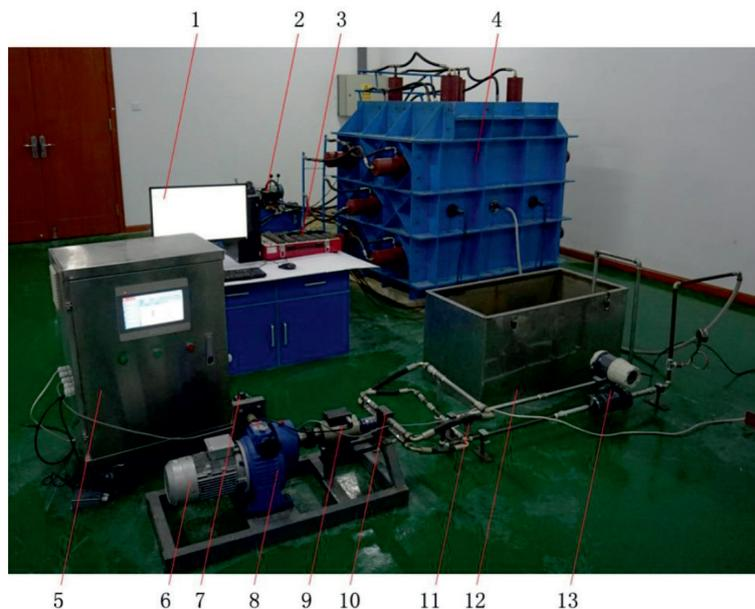
Fig. 7. Model test system: 1. Computer; 2. Hydraulic station; 3. Strain gauge; 4. Model frame; 5. PLC control cabinet; 6. AC motor; 7. Stepping motor; 8. Stepless transmission; 9. Torque sensor; 10. SDU-0.5-23; 11. Pressure sensor; 12. Slurry storage tank; 13. Electromagnetic flowmeter.
