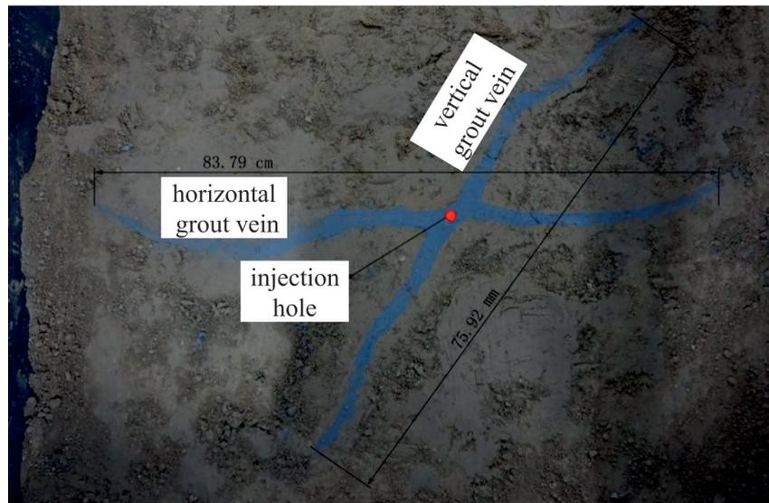
Fig. 13. Removing the soil and expose the grout veins.
