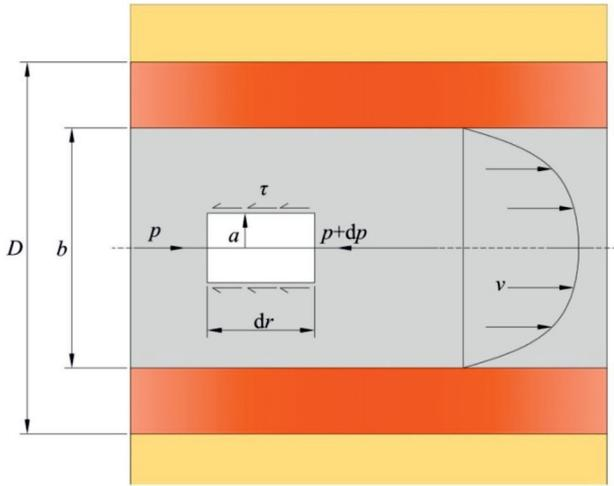
Fig. 5. Propagation model of fracture grouting.
