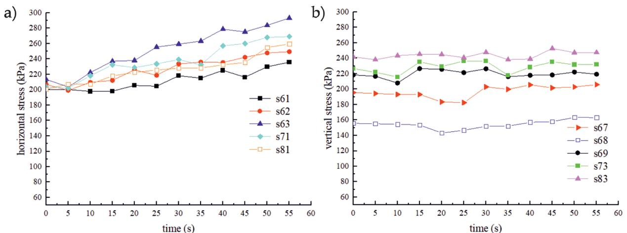
Fig. 12. Stress fluctuation of the second grouting: a) Horizontal stress by second grouting; b) Vertical stress by second grouting.
