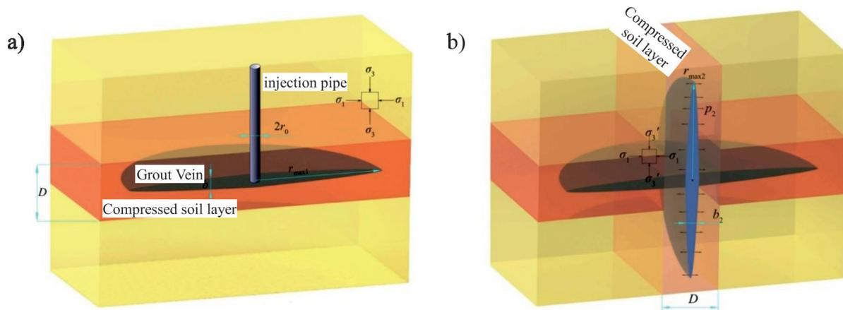
Fig. 2. Propagation model of fracture grouting: Schemes follow another format. If there are multiple panels, they should be listed as: a) Splitting diffusion model of grout vein for preceding grouting; b) Splitting diffusion model of grout vein for subsequent grouting.
