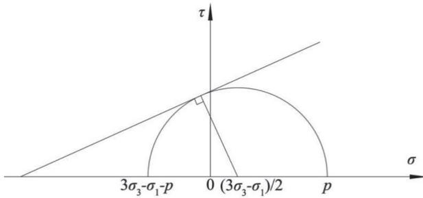
Fig. 4. Stress state when soils breaking near the grouting orifice.
