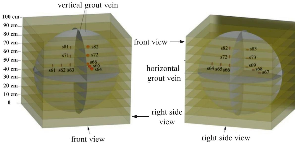
Fig. 9. Three-dimensional layout of earth pressure cells.
