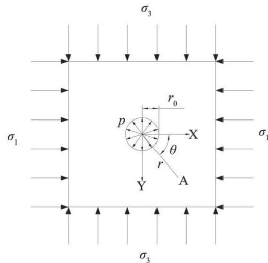
Fig. 3. Stress distribution near the grouting orifice.
