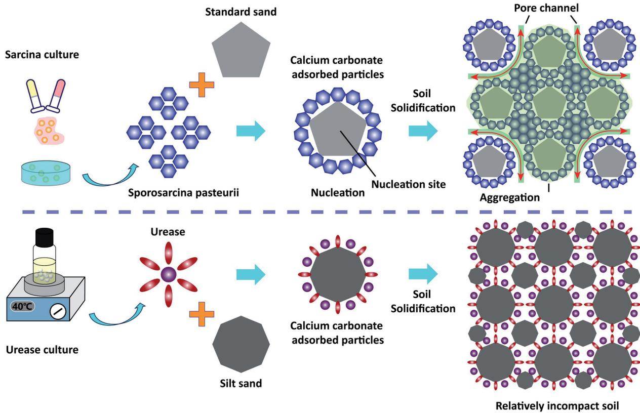
Fig. 8. Reinforcement mechanisms of MICP and EICP methods.
