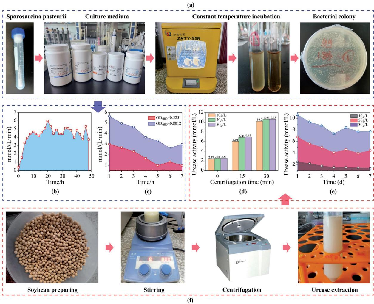
Fig. 1. *Sporosarcina pasteurii* and urease preparation. a) *Sporosarcina pasteurii* culturing; b) Urease activity changes with time; c) Activity variation of *Sporosarcina pasteurii* at 4°C; d) Urease activity under different centrifugation time; e) Activity variation of urease at 4°C; f) Urease culturing.
