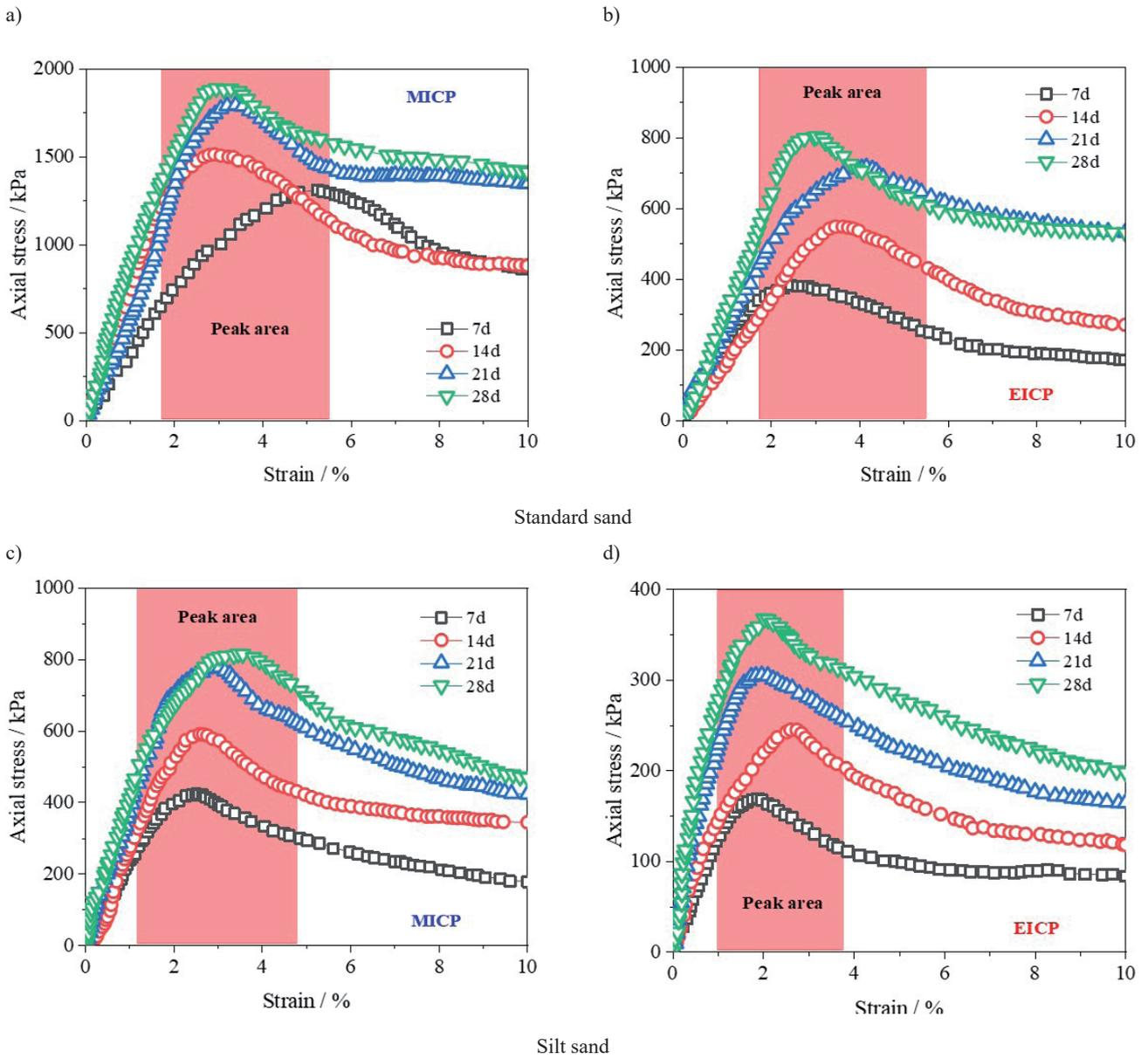
Fig. 3. Compressive strength after solidification respectively with MICP and EICP methods.
