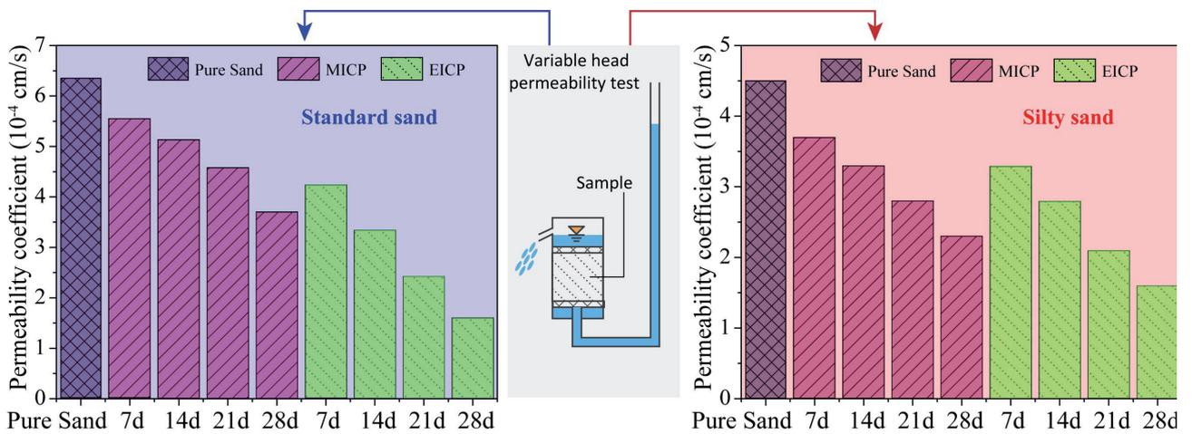
Fig. 4. Changes of permeability coefficient of standard sand and silty sand samples after solidification respectively with MICP and EICP methods.
