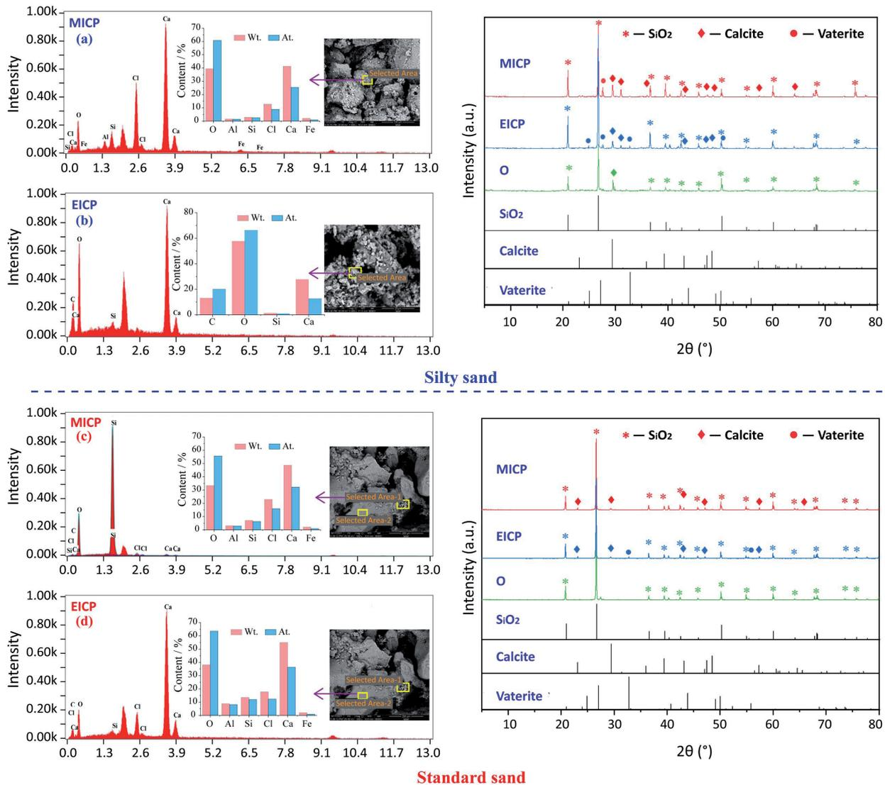
Fig. 7. Changes of the main components of standard sand and silty sand samples after solidification respectively with MICP and EICP methods.
