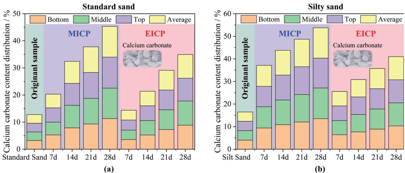
Fig. 5. Changes of the calcium carbonate content of standard sand and silty sand samples after solidification respectively with MICP and EICP methods.
