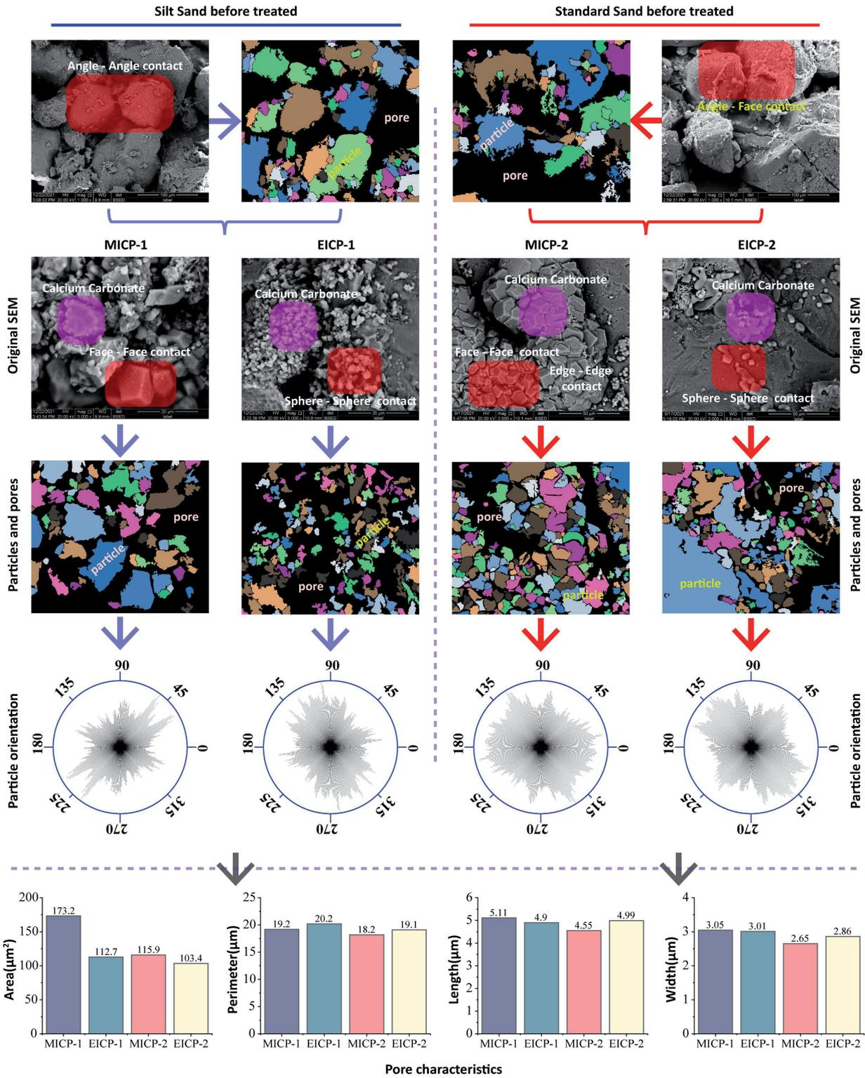
Fig. 6. Changes of the micro-structure of standard sand and silty sand samples after solidification respectively with MICP and EICP methods.
