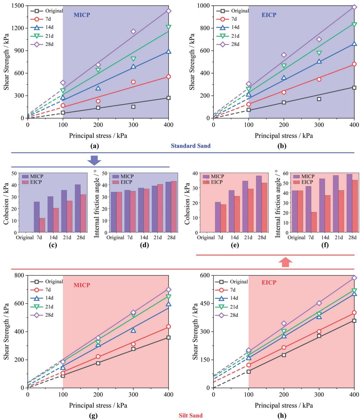
Fig. 2. Shear strength after solidification respectively with MICP and EICP methods.
