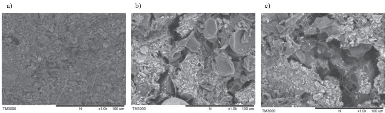
Fig. 7. SEM picture of sludge cake a) Raw sludge; b) Biochar conditioned sludge; c) Biochar and FeCl<sub>3</sub> conditioned sludge.
