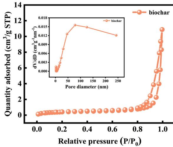
Fig. 1. N<sub>2</sub> adsorption/desorption isotherms of the sludge derived biochar samples.
