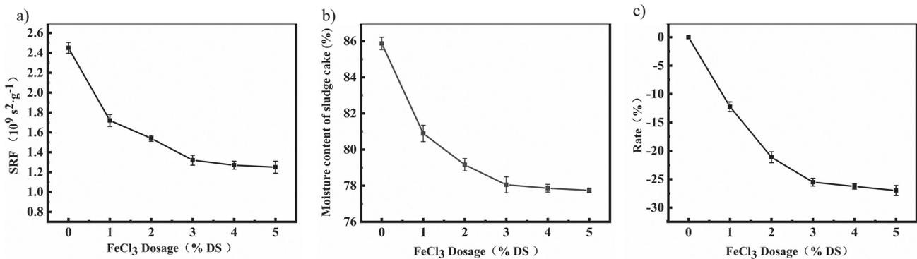
Fig. 3. Selection of the added amount of FeCl<sub>3</sub> a) SRF b) MC c) mass change rate
