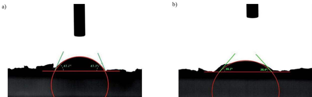
Fig. 2. Contact angle diagram of printing and dyeing sludge and sludge derived biochar a) printing and dyeing sludge b) sludge derived biochar
