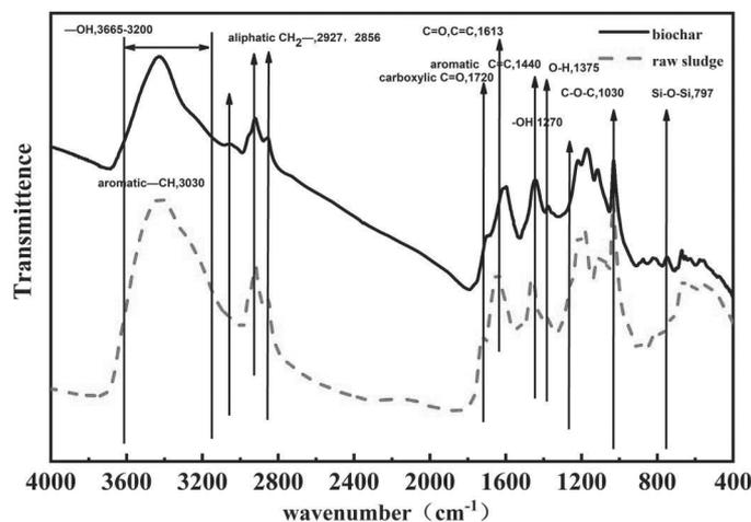
Fig. 9. Infrared spectra of biochar and raw sludge.
