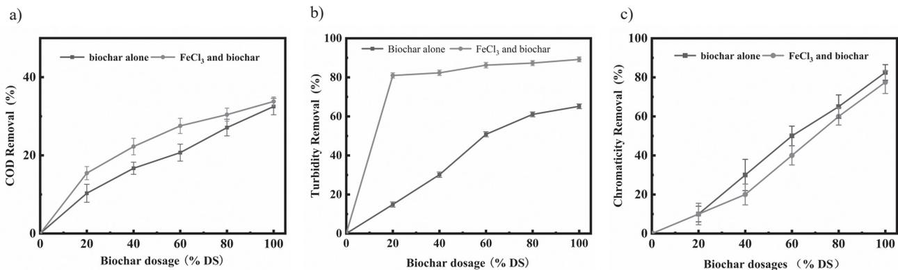
Fig. 6. Effect of Biochar on Supernatant Quality a) COD Removal b) Turbidity Removal c) Chromaticity Removal.
