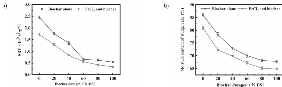
Fig. 5. Effect of biochar dosages on sludge dewatering a) SRF b) MC.
