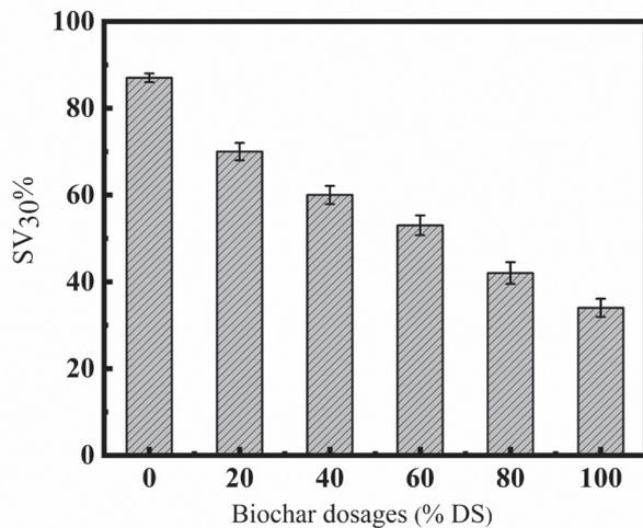
Fig. 4. Effect of biochar dosage on sludge settleability.
