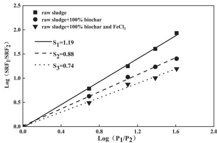
Fig. 8. Effect of biochar on sludge compressibility.
