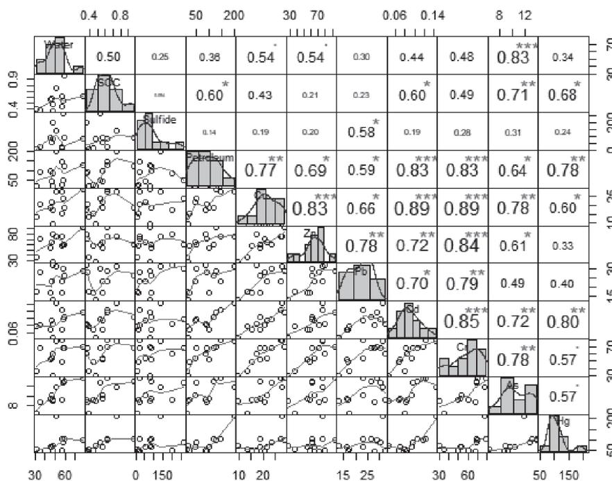
Fig. 5. Pearson correlation coefficient between heavy metals in sediment and other properties.
