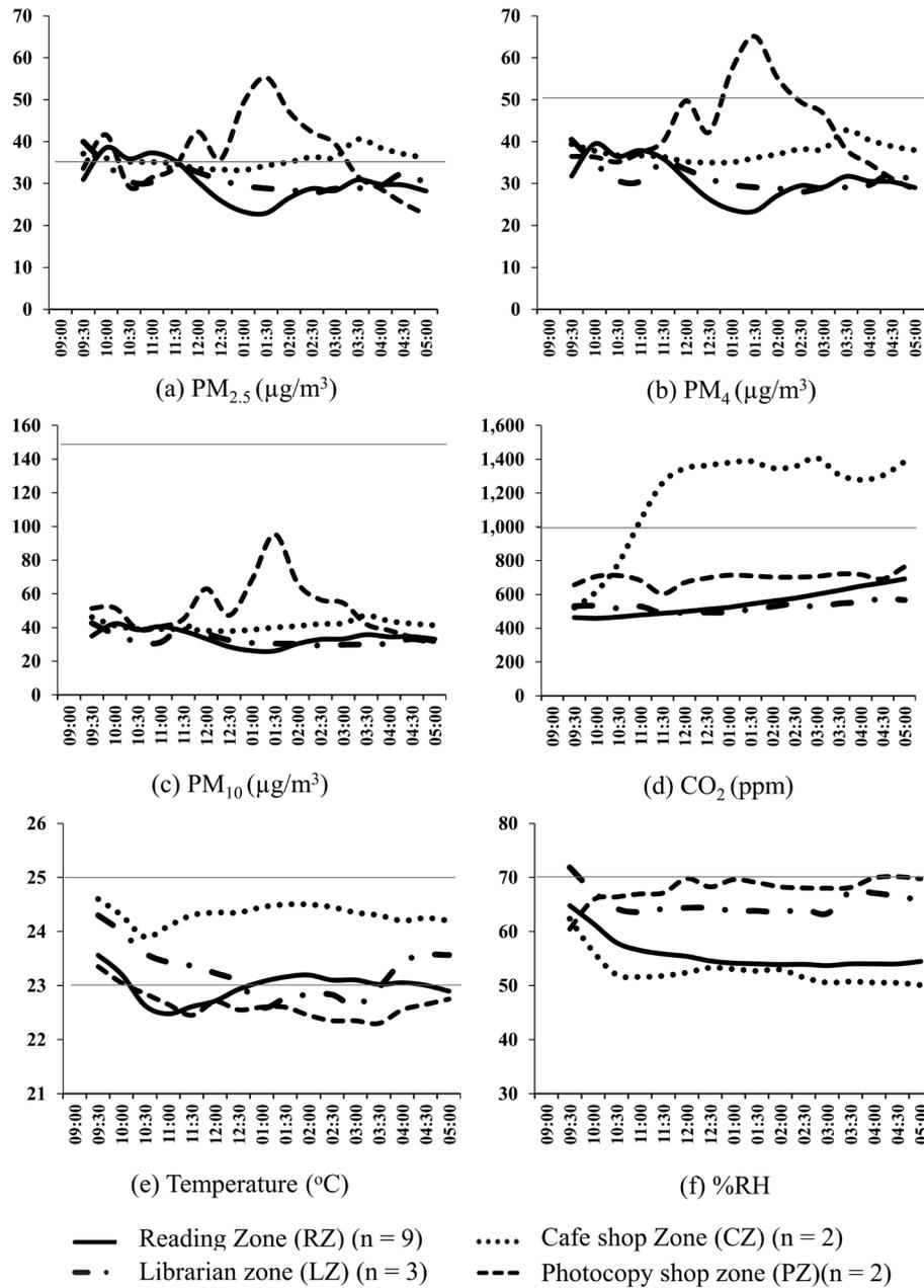
Fig. 2. Temporal variations of indoor parameters: a)  $PM_{2.5}$ , b)  $PM_4$ , c)  $PM_{10}$ , d)  $CO_2$ , e) temperature and f) %RH. Corresponding standard values are shown by the horizontal line (Singapore standards, 2009, 2021) for all parameters, except  $PM_{10}$  for ASHRAE standard 62.1-2010.
