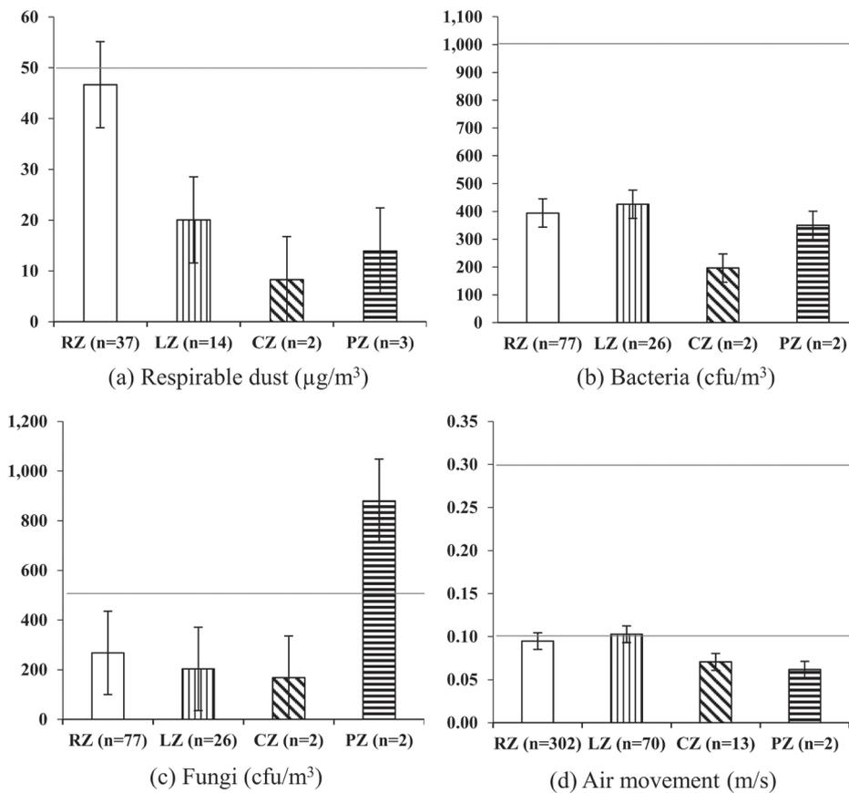
Fig. 1. Average concentration of indoor parameters over the studied period in different zones at the library of a) respirable dust, b) bacteria, c) fungi, d) air movement. Corresponding standard values are shown by the horizontal line (Singapore standards, 2009, 2021).
