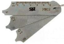
Fig. 12. Universal welder's gauges
