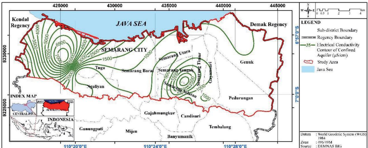
Fig. 8. EC of confined aquifer samples map.
