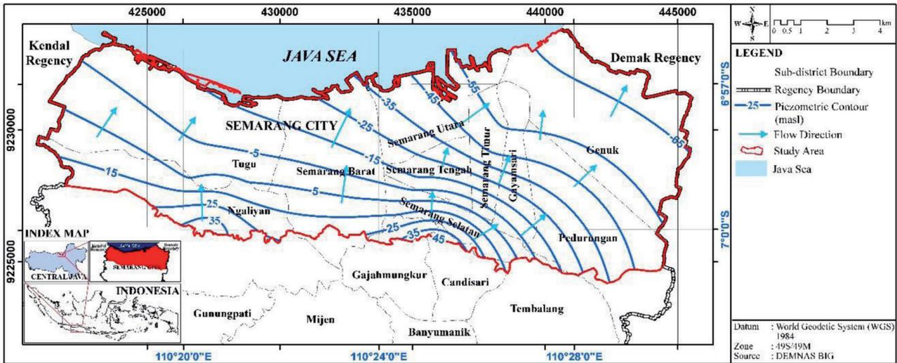
Fig. 7. Piezometric level map.
