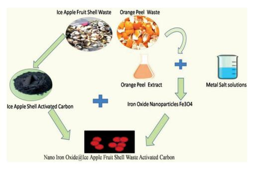
Fig. 1. Schematic presentation of synthesis of IONP@IFSAC
