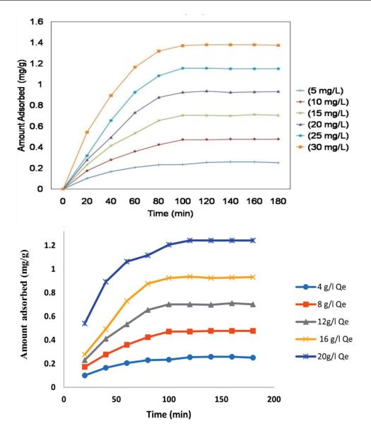
Fig. 3. Effect of time and initial concentration of Pb(II) ions on adsorption
