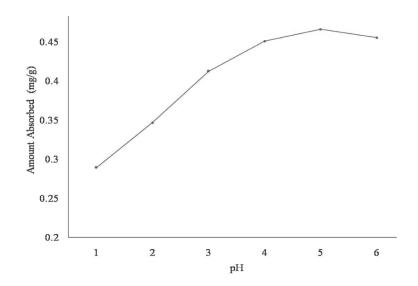
Fig. 5. Effect of pH on adsorption of Pb(II) ion
