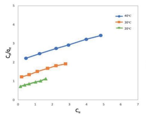
Fig. 6. Langmuir plots for Pb(II) ion removal at different temperatures
