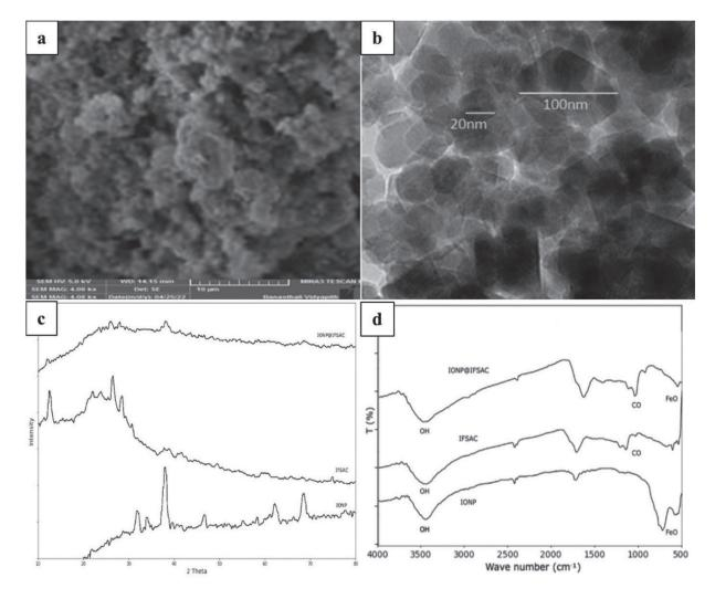
Fig. 2. Characterization of IONP@IFSAC by a) SEM b) TEM c) XRD d) FTIR
