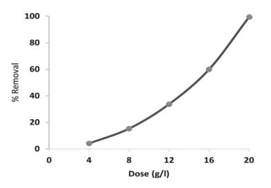
Fig. 4. Effect of adsorbate dose on Pb(II) ions adsorption
