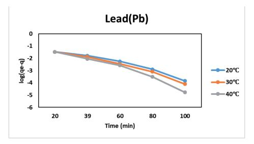
Fig. 7. Freundlich Adsorption for Pb(II) metal ion removal at different temperatures
