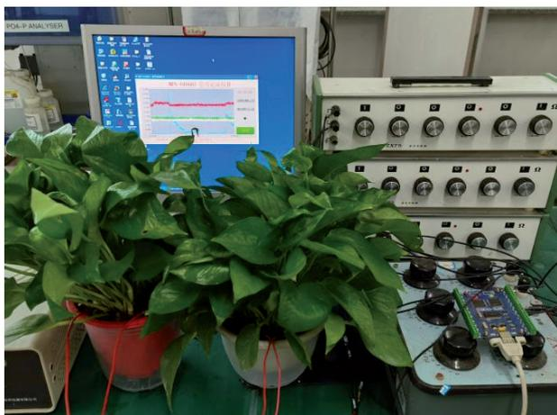
Fig. 1. Experimental system of PMFC.
