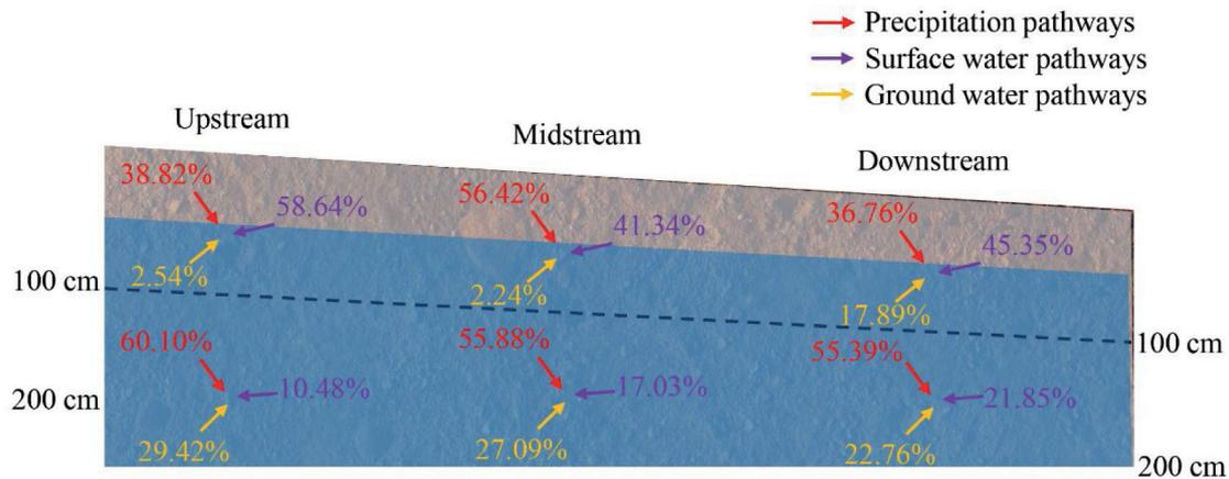
Fig. 8. Analysis of the source of soil-water in gully.
